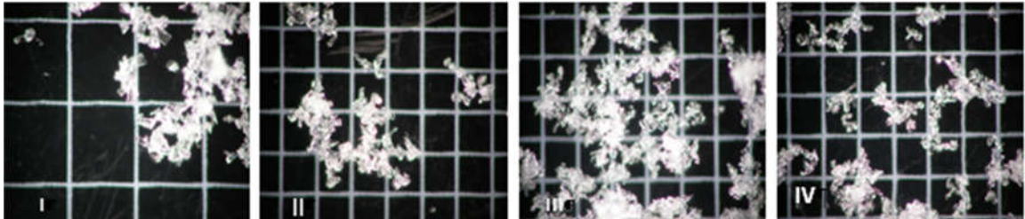
Figure 48: Radiation recrystallization photos from Yellowstone Club ski patrol at (I) 0 cm, (II) 1 cm, (III) 2 cm, and (IV) 3 cm below the surface taken on January 11, 2011.
