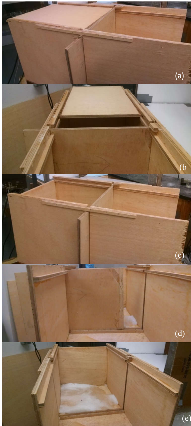
Figure 4: The snow box used in the lab (a) Shows the box with the sliding front and sliding top closed, (b) is the top sliding off, (c) is the box with the top removed, (d) is the front of box being removed, and (e) is the box without its front or top.
