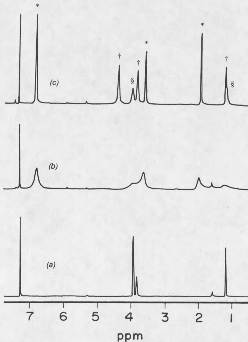
Figure 17. NMR spectra at 250 MHz of [(\text{NBD})\text{RhCl}]_2 in \text{CDCl}_3 at 25^\circ\text{C} : (a) rhodium complex alone; (b) rhodium complex and NBD (1:4 molar ratio); (c) same as part b but at -55^\circ\text{C} ; (*) resonances attributed to uncomplex NBD ; (†) resonances of monomeric complex (\text{NBD})_2\text{RhCl} ; (§) resonances of the dimeric complex [(\text{NBD})\text{RhCl}]_2 .
