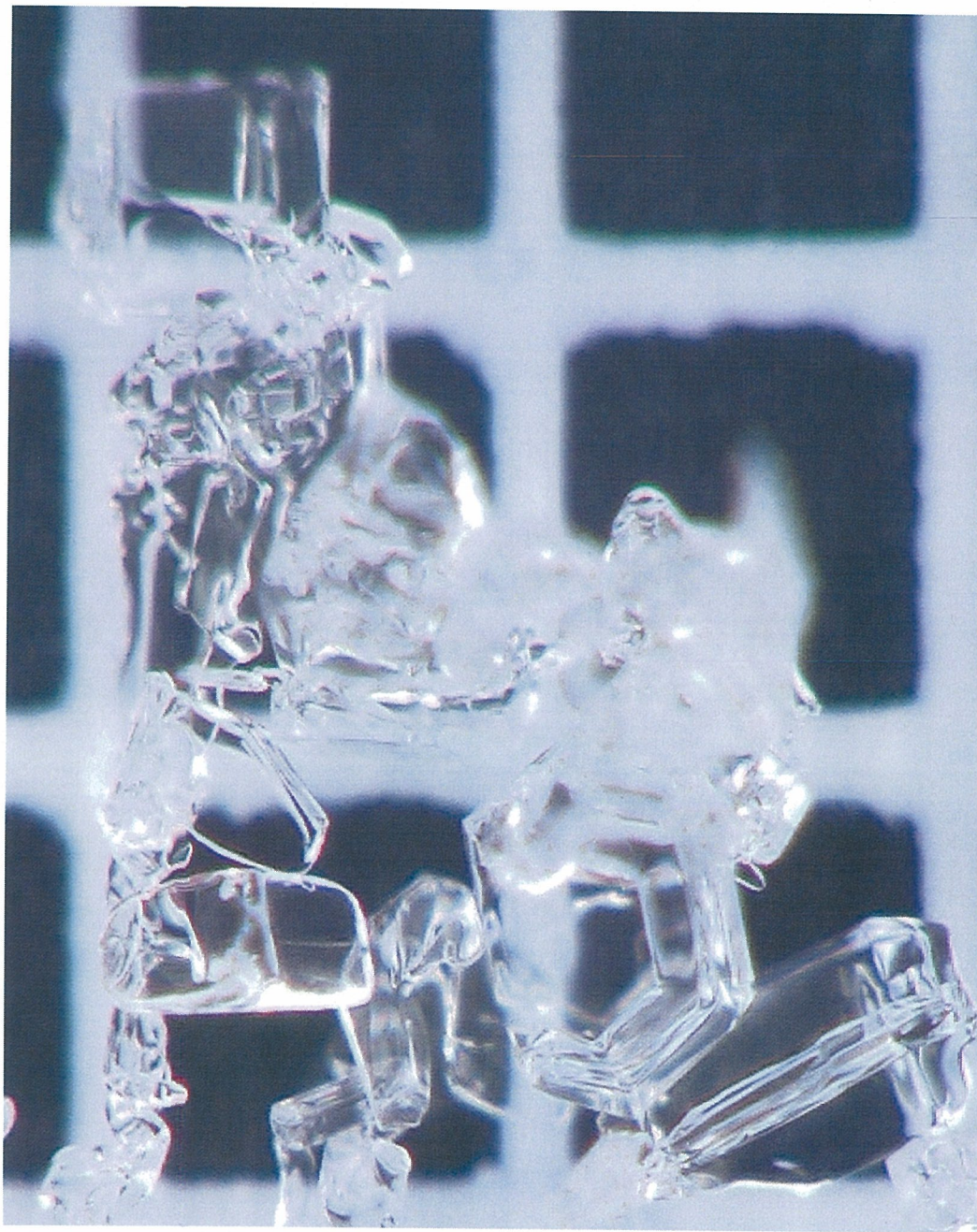
Figure 4.42: One mm faceted crystals harvested from the north-facing study site on 13 March 2004. These crystal would be classified by Colbeck et al. (1990) as type 4a, solid faceted particles.
