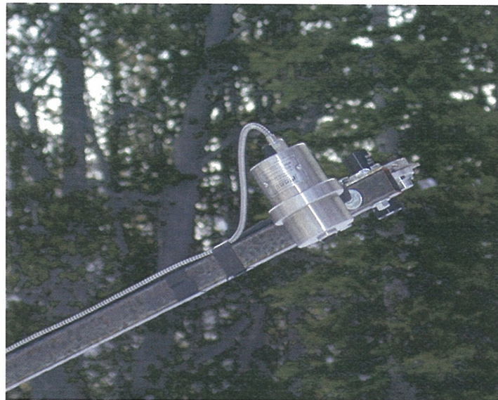
Figure 3.6: The thermocouple array placed at slope parallel in the snow with the 0.10 m and 0.05 m above the snow surface thermocouples visible and the snow surface thermocouple at the snow air interface border.
