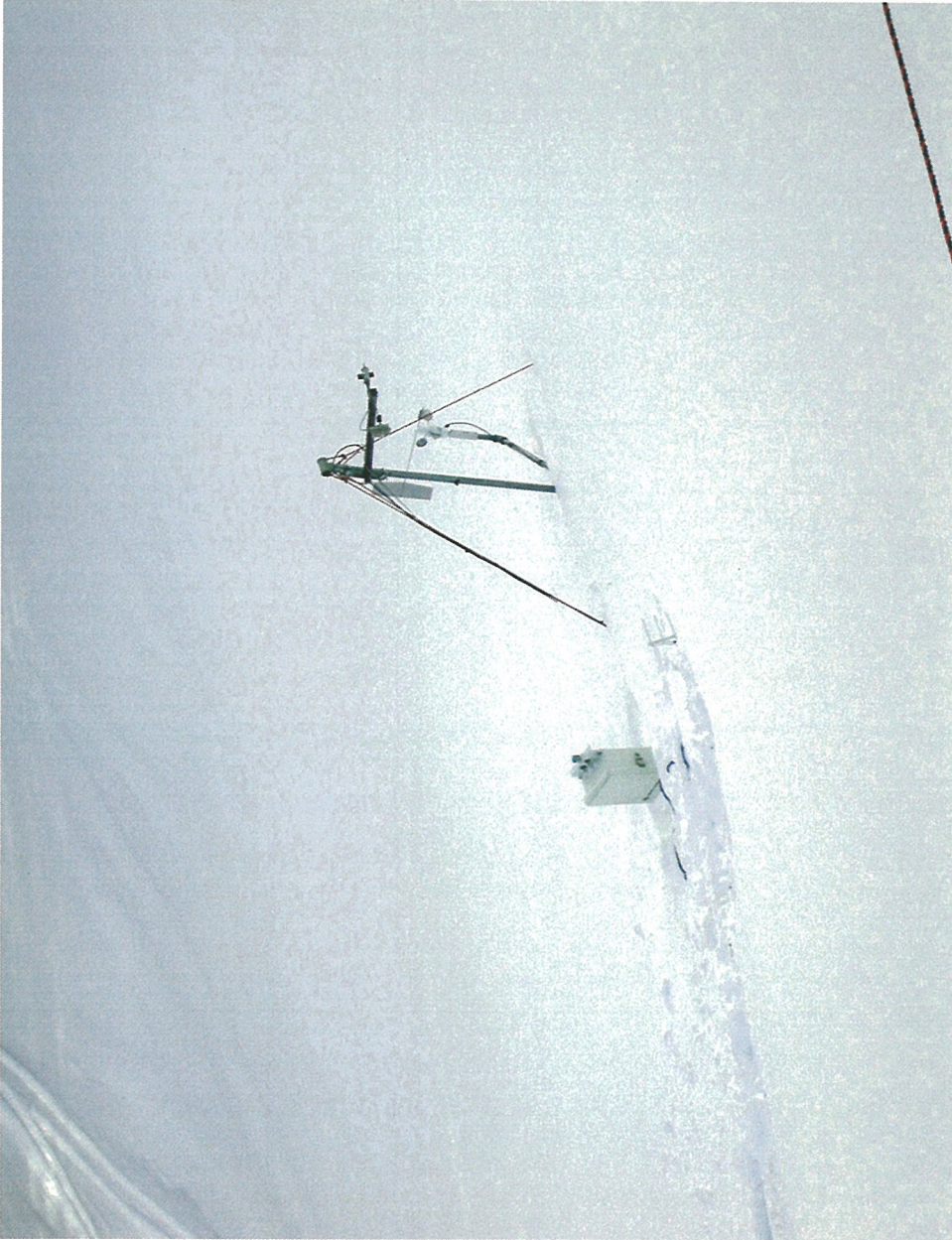
Figure 3.5: The north study site in the winter, showing the anemometer with its movable arm and the pyranometers. Also in view are the datalogger and the thermocouple array (center of photograph).
