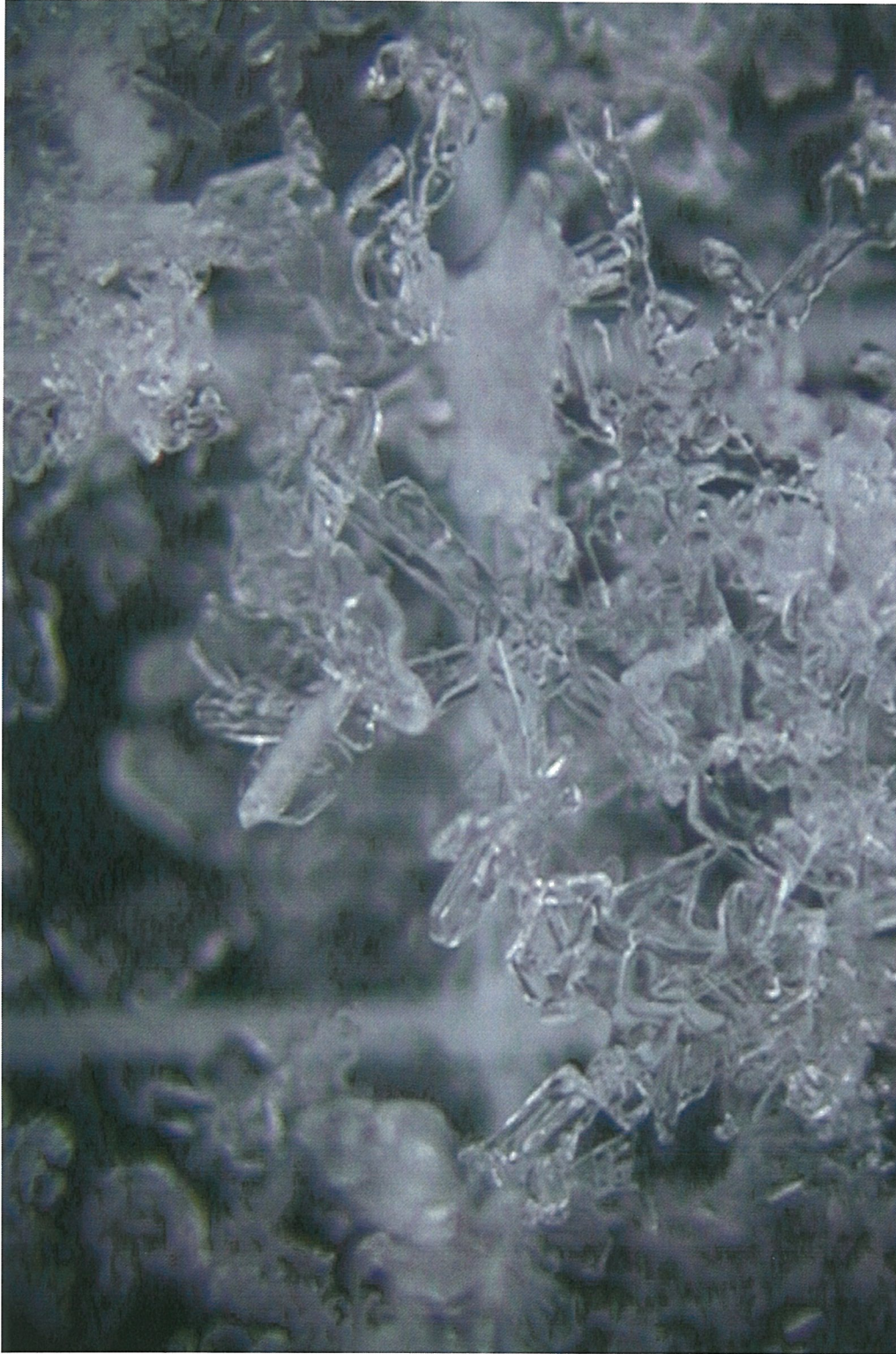
Figure 4.48: One to two mm stellar and broken particle crystals harvested from the south-facing study site on 9 February 2004. The crystals are classified by Colbeck et al. (1990) as type 1d, stellar dendrite, and 2a, broken.
