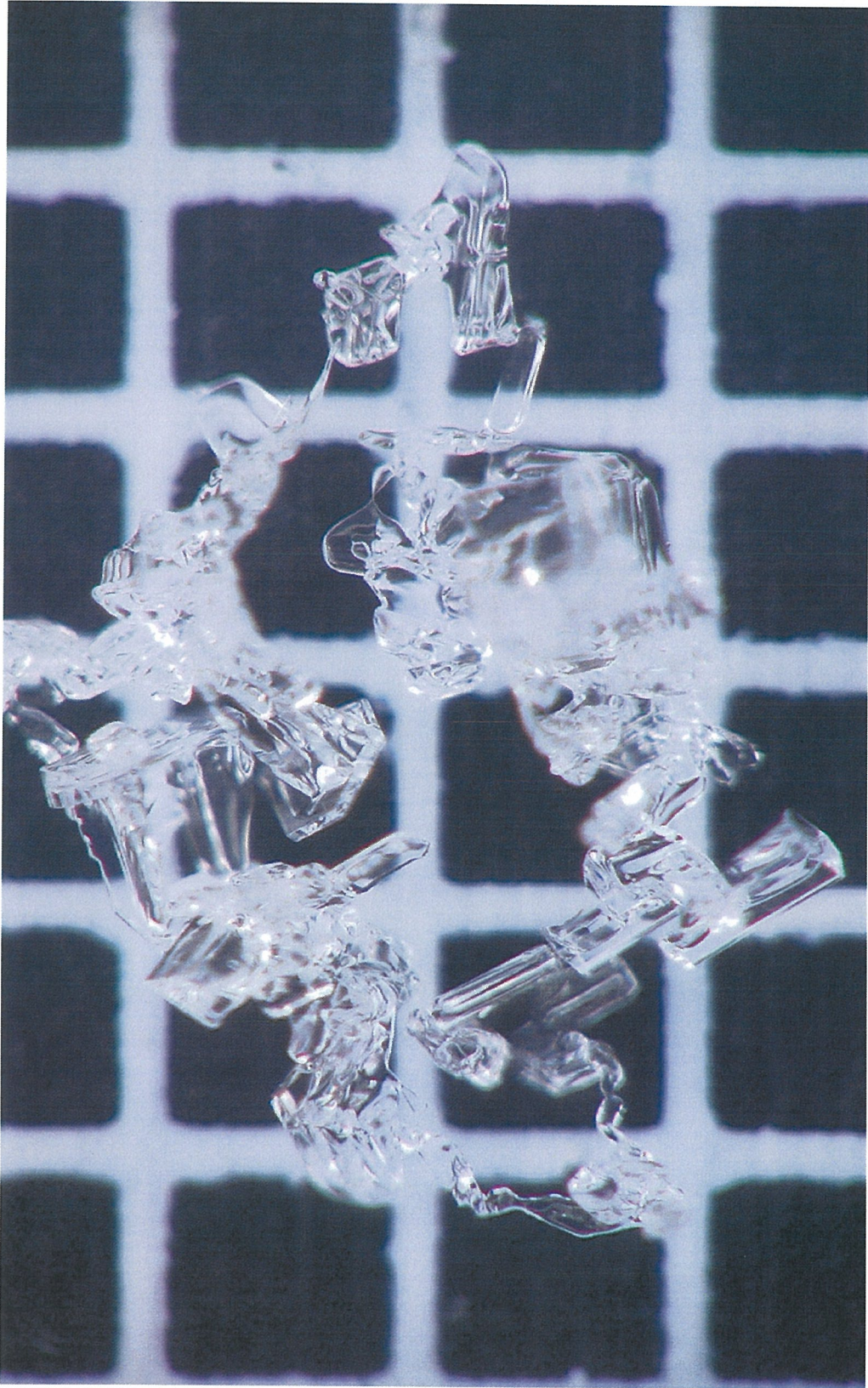
Figure 4.43: One mm near-surface faceted crystals harvested from the south-facing study site on 13 March 2004. These crystals would be classified by Colbeck et al. (1990) as type 4a, solid faceted particles.
