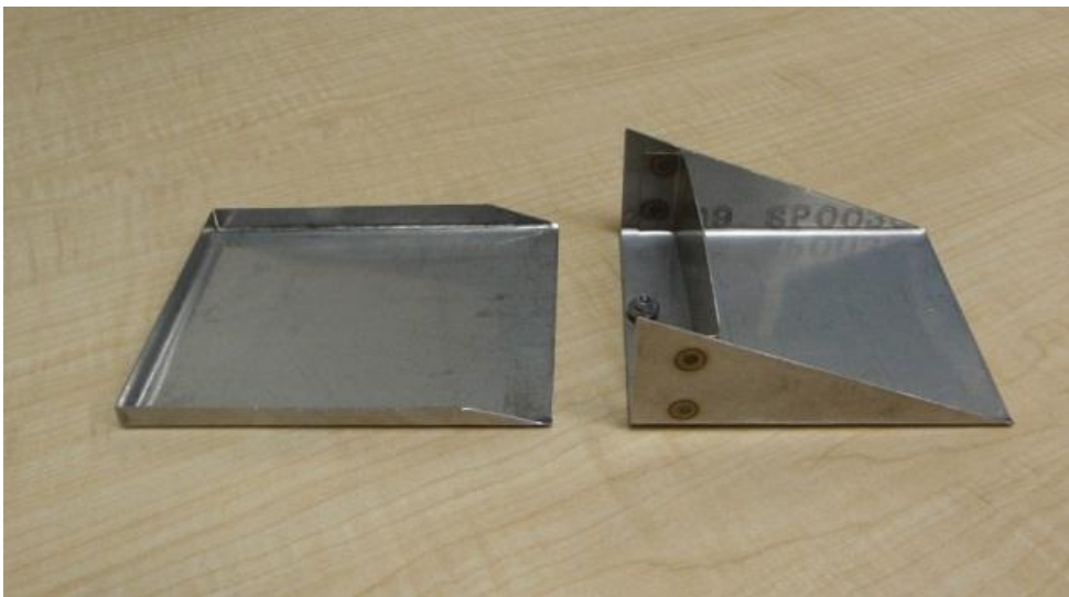
Figure 9: The 200 cm 3 triangular cutter with lid. The triangular base is pushed into a snow layer and the lid is slid over the top to cut the snow.
