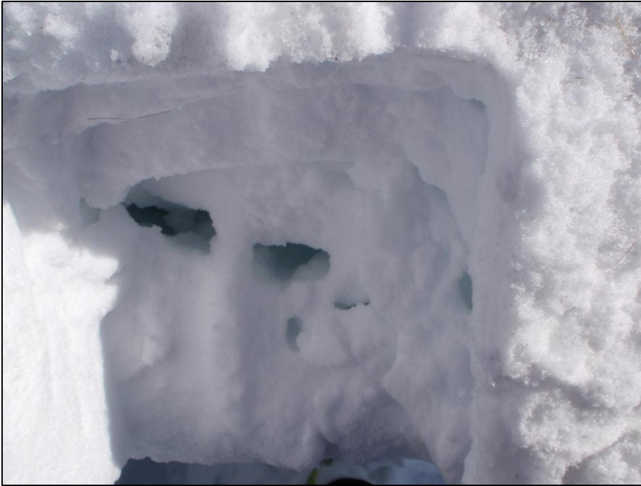
Figure 30: Example of discontinuities found within the snowpack looking down into the snowpack where a portion of the top layers of snow has been removed. These holes were found while excavating a pit 1 m from the blast center.
