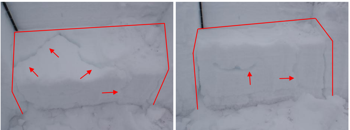
Figure 32: Post-blast ECT column 1 m from the blast center showing top view on left and facing view on right. The top portion of the column above the failure layer has been removed. Arrows highlight cracks and holes that were both inside the snowpack and visible from the front when the column was excavated.
