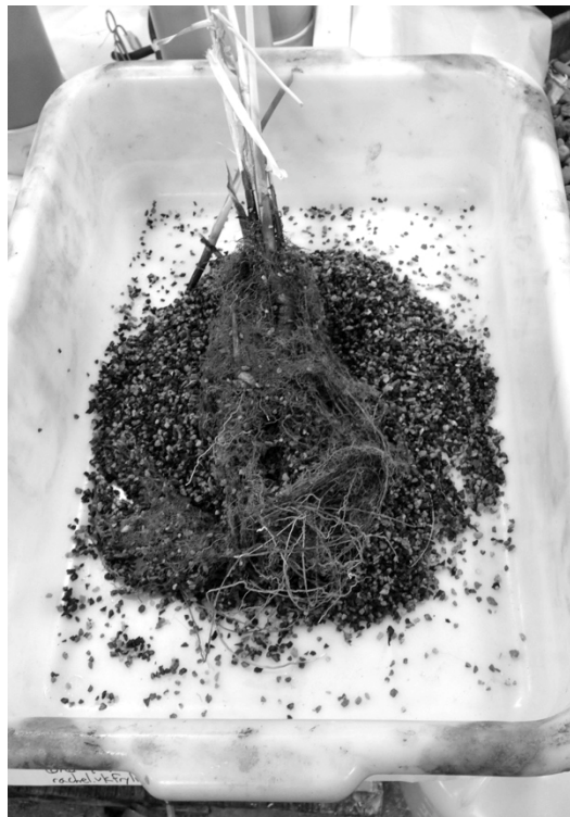
Figure 4.2. Image of destructive sampling technique. S. acutus plant is pictured removed from the batch column in horizontal stratification for sampling of root and gravel while in secondary containment for E. coli O157:H7 handling procedure.
