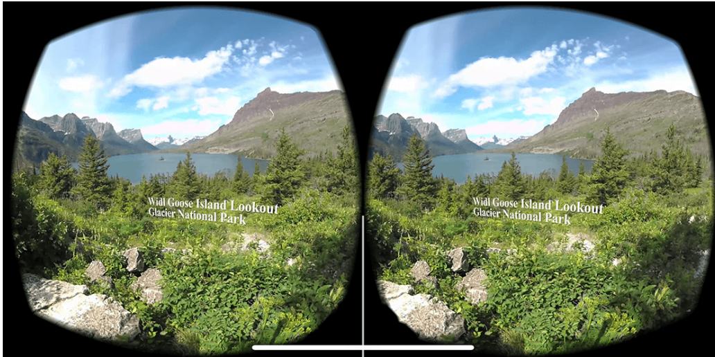
Figure 4. YouTube Google Cardboard Playback. Viewing the 360 video through YouTube's app on smartphones with the Google Cardboard. The screen is split into two playback videos that optically merge when viewing through the magnification lenses.
