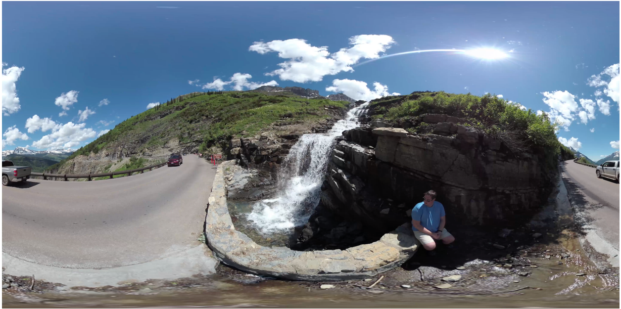
Figure 2. Equirectangular 360 video. The equirectangular video distorts objects at the top and bottom of the sphere in a rectangular projection. Notice that a vehicle split in half along the left and right edge of this rectangle. The edges of this equirectangular video will be digitally joined to create a globe-projection out of this flat surface area.
