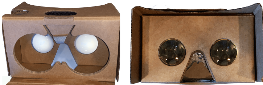
Figure 3. Google Cardboard. The low-tech VR goggles place a smartphone against the front (left), and viewers watch through the lenses on the back (right).
