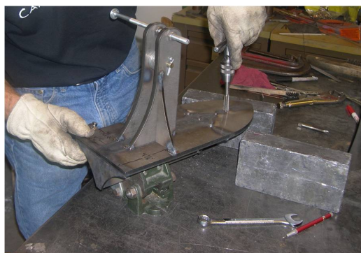
(b) Assembling the trolley
