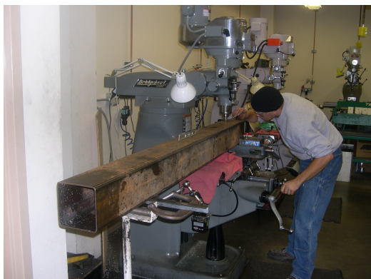
(a) Machining the crane mast
