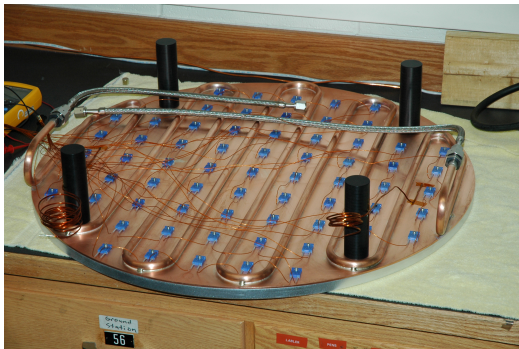
(c) After installing the thermocouples and liquid Nitrogen lines
