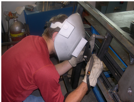
(a) A student welds parts of the table together
