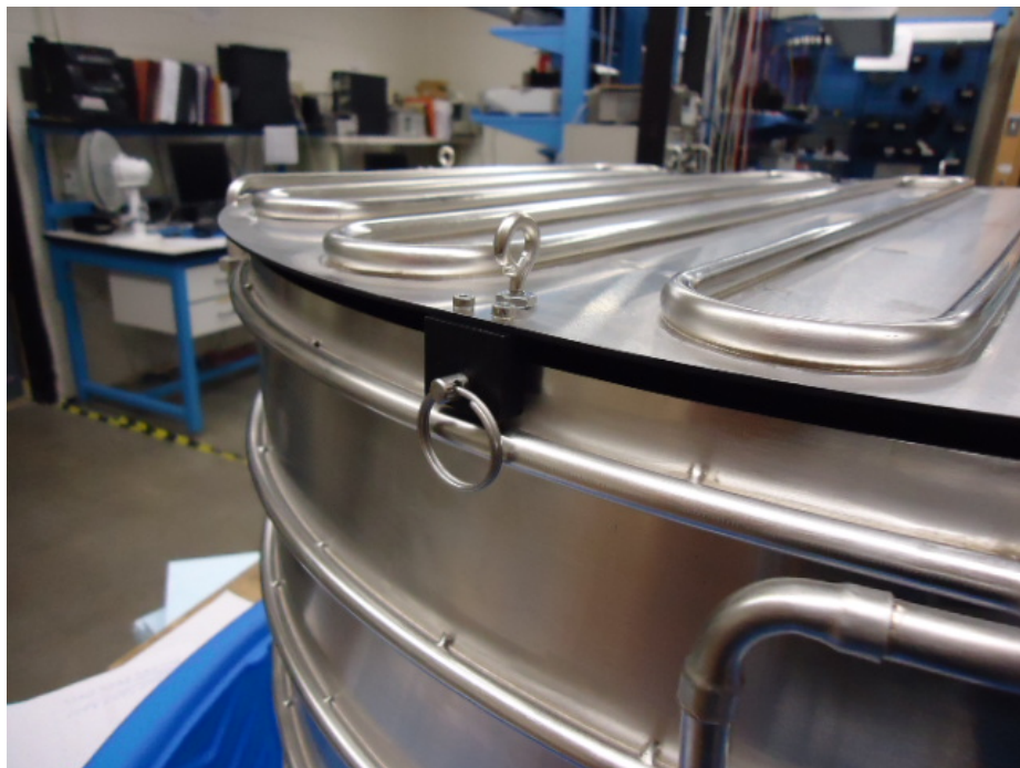
Figure 5.2: Thermal Shroud Insulator Assembly
