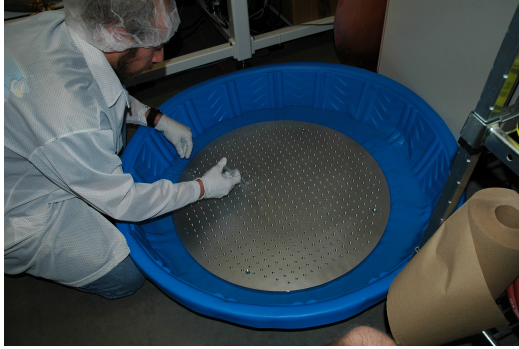
(a) Cleaning the base plate in an alcohol bath
