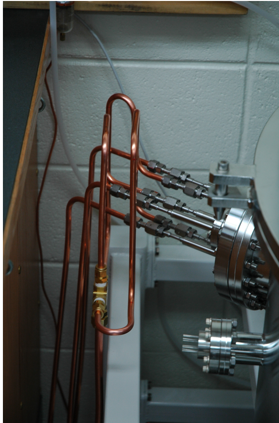
(b) Copper Tubing Connecting to the Chamber
