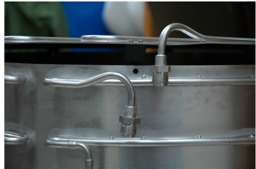
(b) Shroud Alignment Vertical Mismatch
