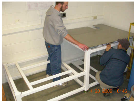
(b) Students installing the table in the lab after powder coating
