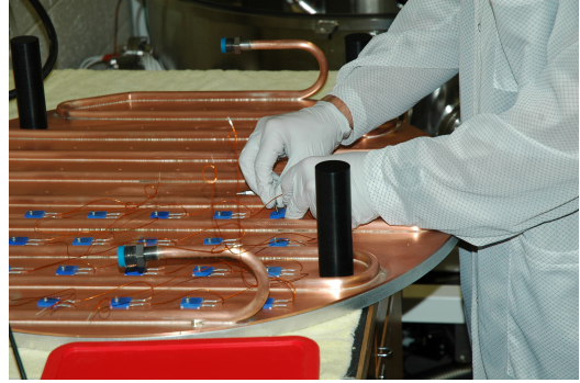
(b) Assembling the heaters to the Aluminum and Copper plates
