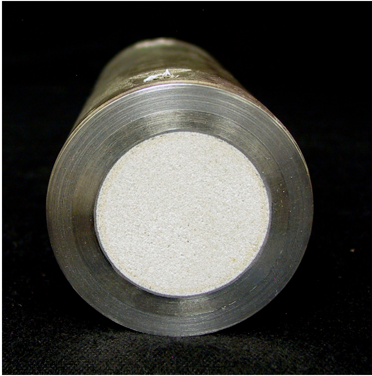
Figure 8.1: An end view showing the thickness of the casting metal, allowing high pressures to be applied while maintaining linear flow.
