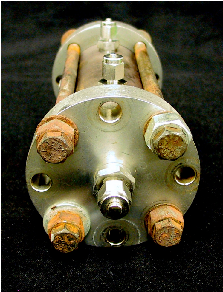
Figure 8.2: The inlet of the core holder.
