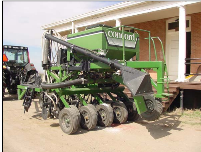
Figure 1. Research-scale Concord air drill system equipped with computerized variable rate technology. Individual plot observations will consist of 10, 50-foot rows on fixed 12-inch row spacing.
