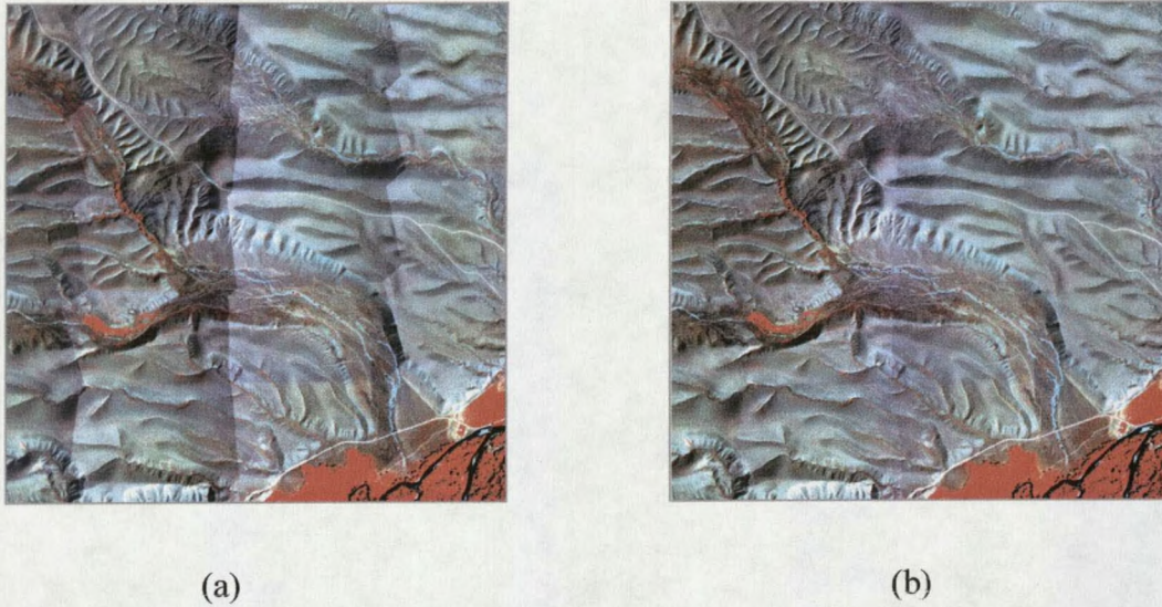
Figure 5. Mosaicked ADAR 5500 image of E. esula site captured on 7 August 1999 in Madison County, Montana showing (a) within and between scene brightness gradients and (b) after processing with DIME TM color balancing software. Bands 4 (780-920 nm), 3 (610-700 nm), and 2 (520-610 nm) are displayed as red, green, blue, respectively.
