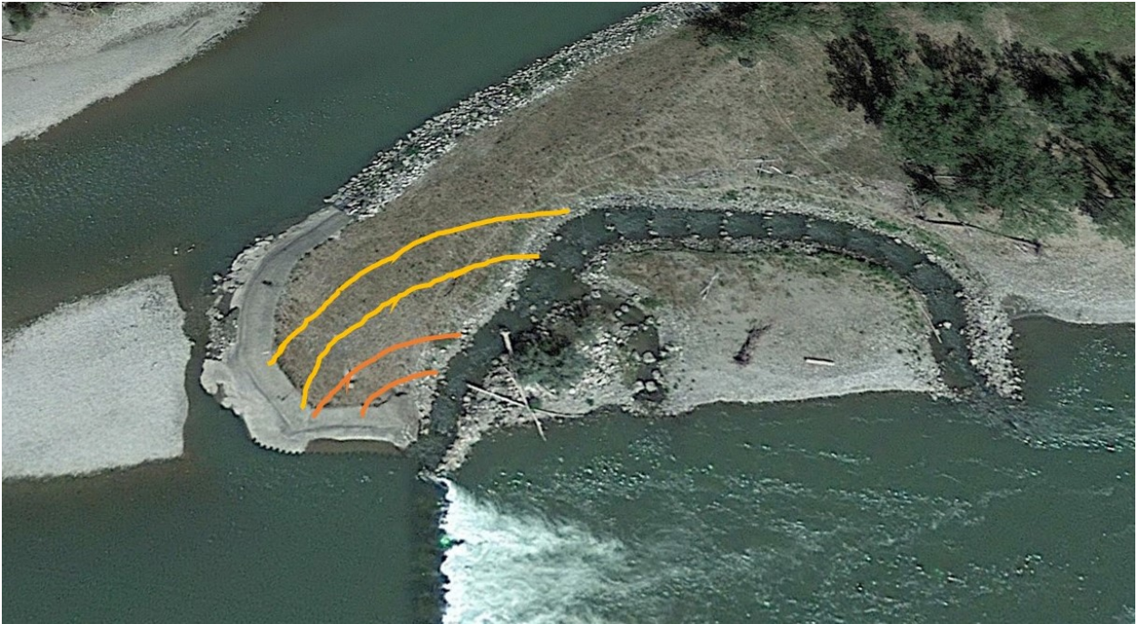
Figure 16. Diagram outlining two potential locations of a secondary nature-like exit channel that could be constructed at the nature-like fishway at Huntley Diversion Dam, Yellowstone River, Montana, to provide an alternative upstream passage route for fish during high discharges when turbulent, high velocity water is present near the existing exit. A secondary exit channel could contain boulders and other roughness elements similar to those in the existing channel.
