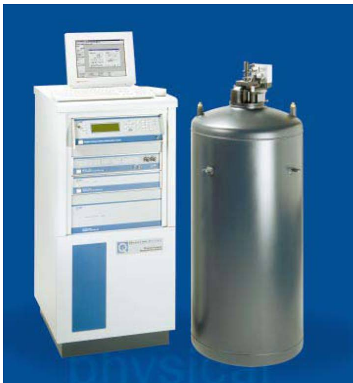
Figure 2.6: The PPMS control system along with the helium dewar where the superconducting magnet and magnetic probes measure the magnetic properties.
