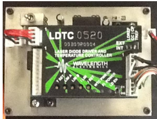
Figure 6 Image of the LDTC0520 mounted on the relay circuit PCB.
