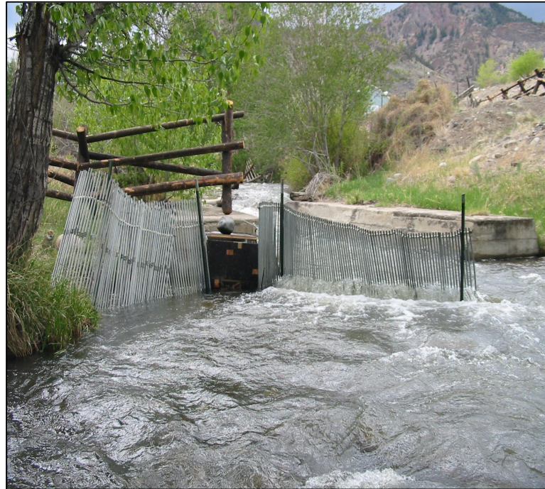
Figure 32. Picture of the tagging trap (trap #1) and fences that direct fish to the trap opening.
