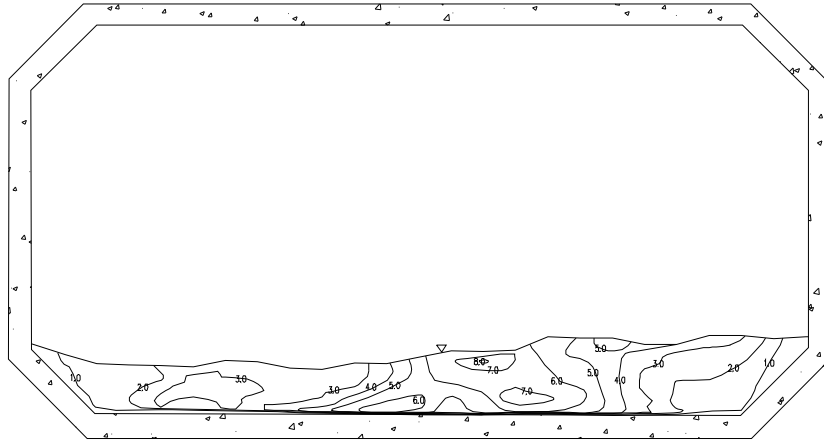
Culvert #1; May 26, 2004; Velocity Contours; Contour Interval = 1.0 ft/s; Discharge = 43.13 cfs; View Downstream; Culvert Width = 12.0 ft; Culvert Height = 6.0 ft. Instrument = Pygmy Meter.
