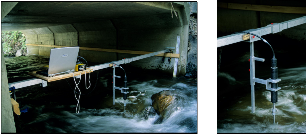
Figure 4. Photograph of the inlet region of Culvert 2 and the ADV harness and meter.
