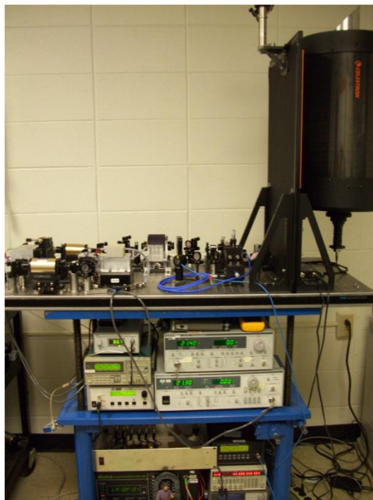
Figure 40 Picture of the second generation DIAL instrument. The transmitter is on the 2'x4' optical breadboard and the receiver is attached to a vertical breadboard where the output beam is transmitted coaxially with the telescope via two 45 degree turning mirrors. All of the instrument electronics are on the shelf below the instrument.
