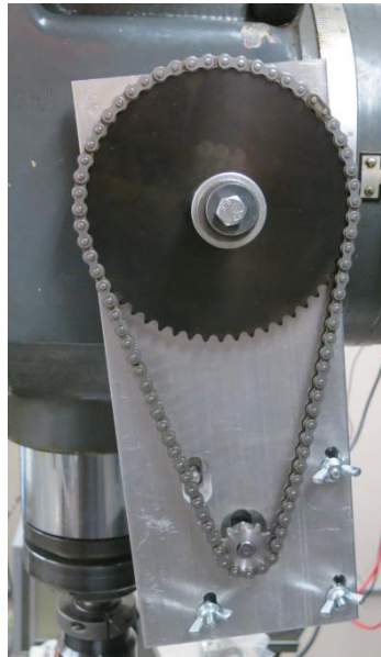
Figure 24: The torque from the motor was amplified.
