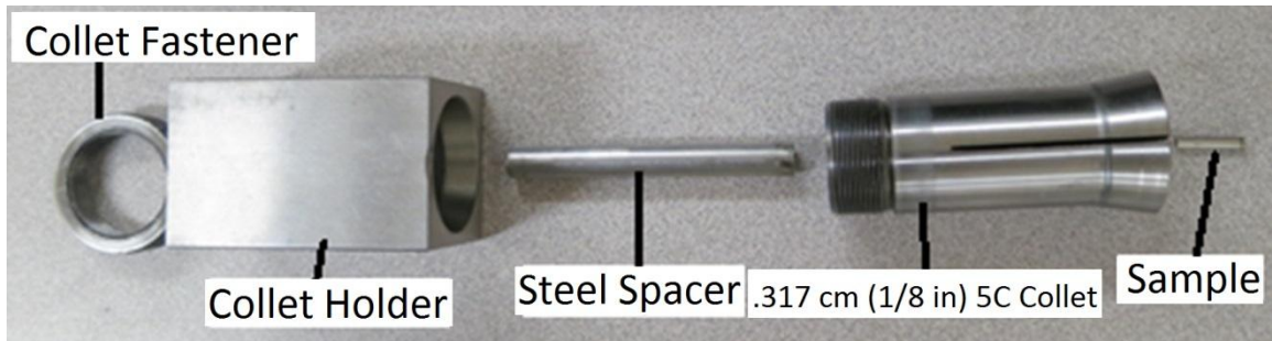
Figure 30: Collet assembly.
