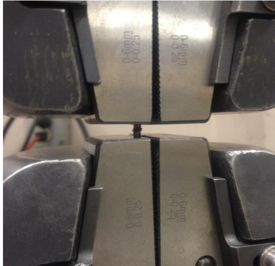
Figure 44: A sample is loaded in the Instron. This was where fracture testing was performed.
