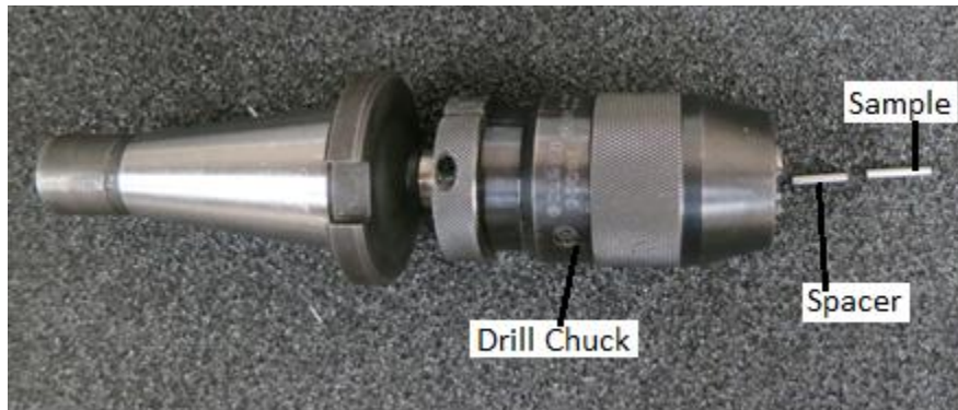
Figure 32: Assembly to hold the upper sample in the drill chuck.
