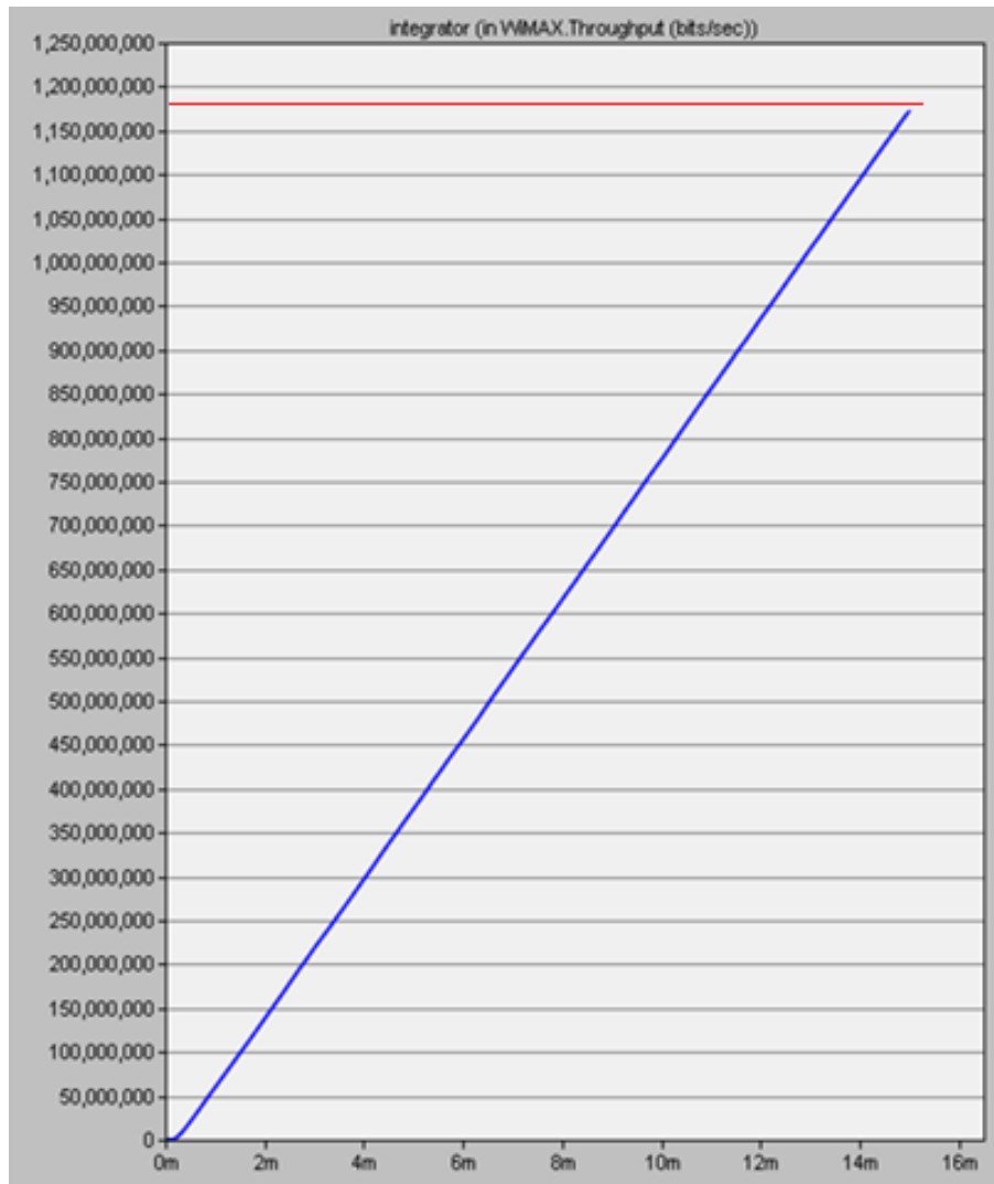
Figure 6.15 – Total throughput (BS) for large scenario after implementing BFS+BHNB and IALU methods with directional antennas.
