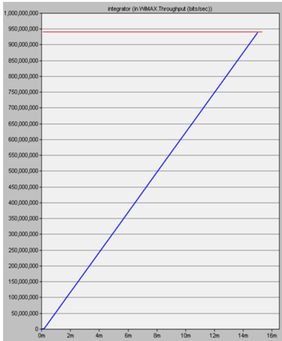
Figure 6.14 – Total throughput (BS) for large scenario without implementing BFS+BHNB and IALU methods with directional antennas.
