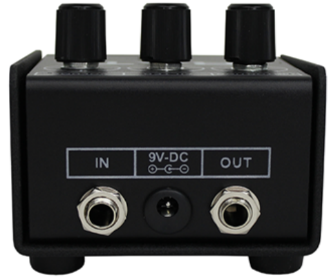
(b) Rear view of ProCo Rat 2 guitar pedal. The monophonic input and output signals are passed via 1/4" tip-sleeve connections.
