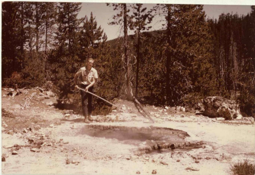
Figure 1. The author using an extension pole with bucket to collect a water sample from station 2.
