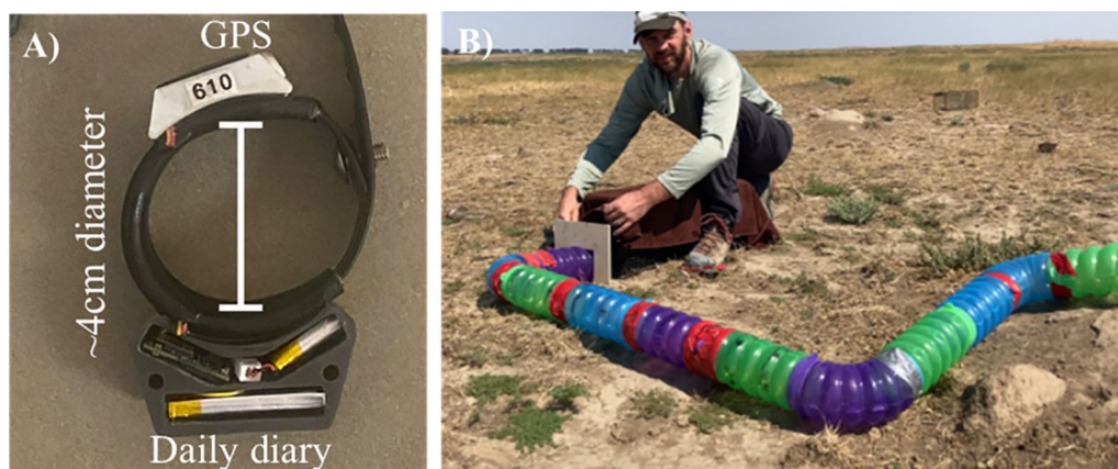
Fig. 1 Technology and apparatus used to assess dead-reckoning potential for prairie dogs. A Photo of the logging system deployed on prairie dogs; B with example of constructed tube run with trap connected
