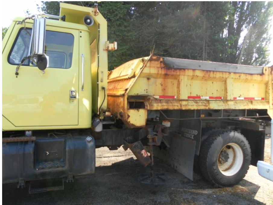
Figure 32: Side-discharge salt spreader showing extensive corrosion.
