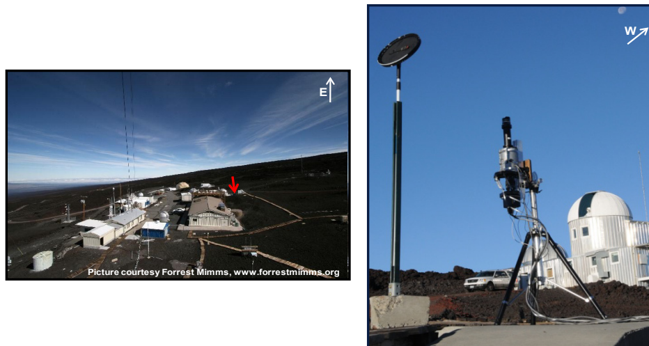
Figure 8: (L) Mauna Loa Observatory as viewed from the CO 2 monitoring tower facing east (photo by Forrest Mims III). (R) Instrument deployed along a roughly East-West line with adjustable sun occulter to the left of the image (Photo by J. A. Shaw).
