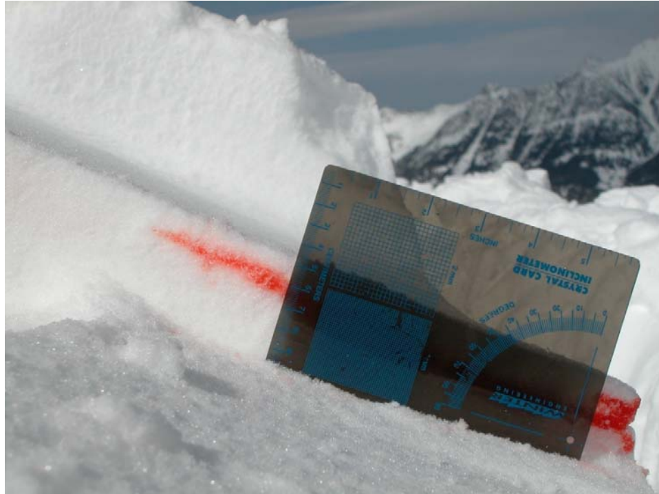
Figure 24: Transition that impeded water shown by red dyed water at interface of 1 finger hard buried wind slab over a 4 finger hard layer of mixed faceted grains.
