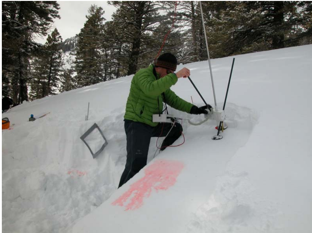
Figure 16: Karl Birkeland of the U.S. Forest Service National Avalanche Center completing SMP measurements upslope of the dyed area.
