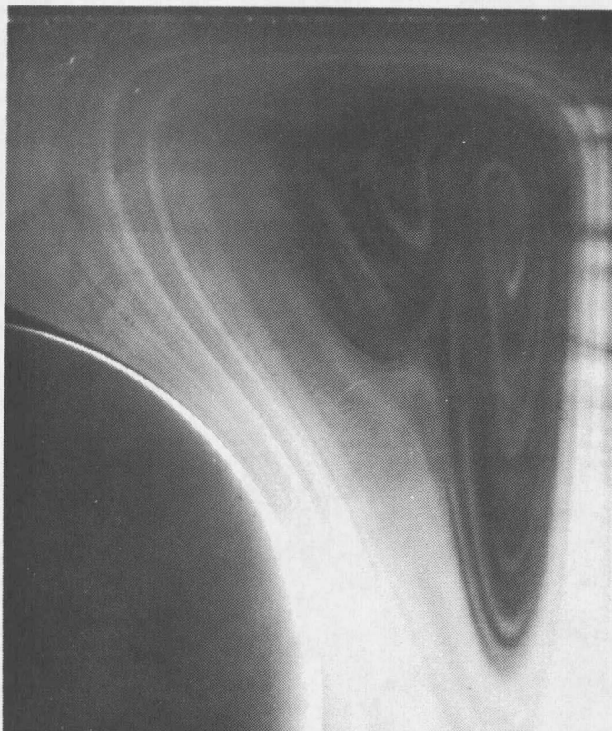
Figure 4.8 Flow Pattern in the Upper Central Region of the Perpendicular Vertical Plane for
