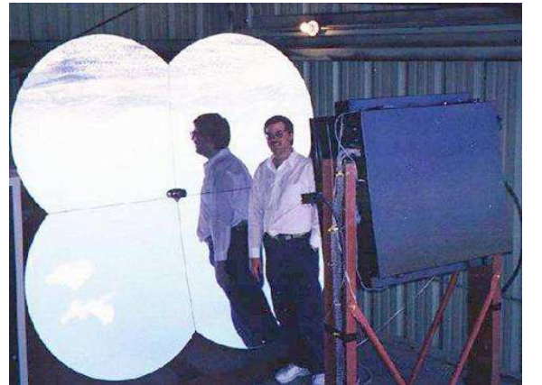
Figure 2.2: A single detector: a mirror and array of photomultiplier tubes.
