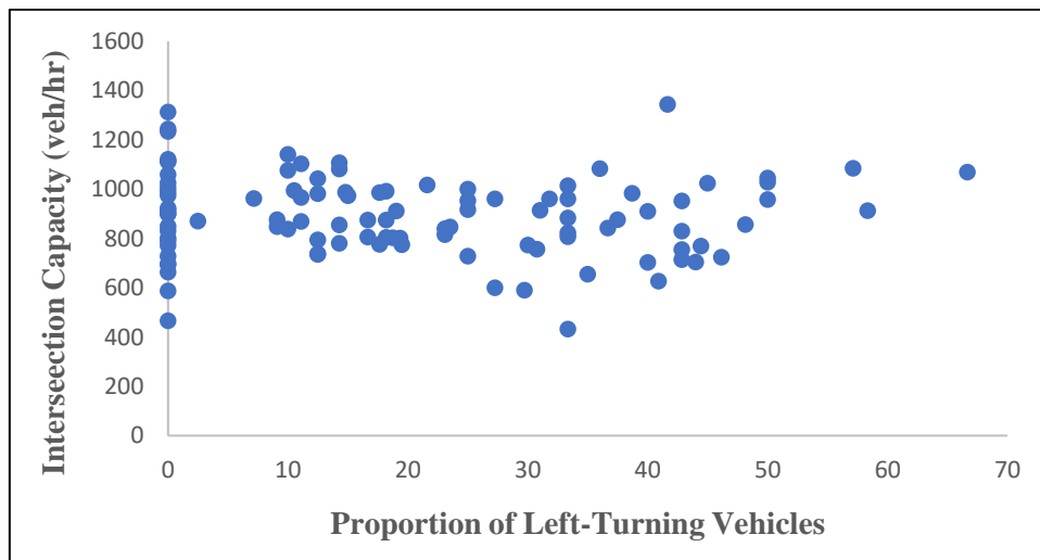
Figure 9. Intersection Capacity versus Proportion of Left-Turning Vehicles
