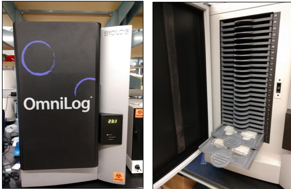
Figures 7 and 8: Images showing the Omnilog instrument used for the substrate utilization experiment. On the left is the instrument set at ambient temperature during the experiment, and on the right is the inside of the Omnilog loaded with Ecoplates.
