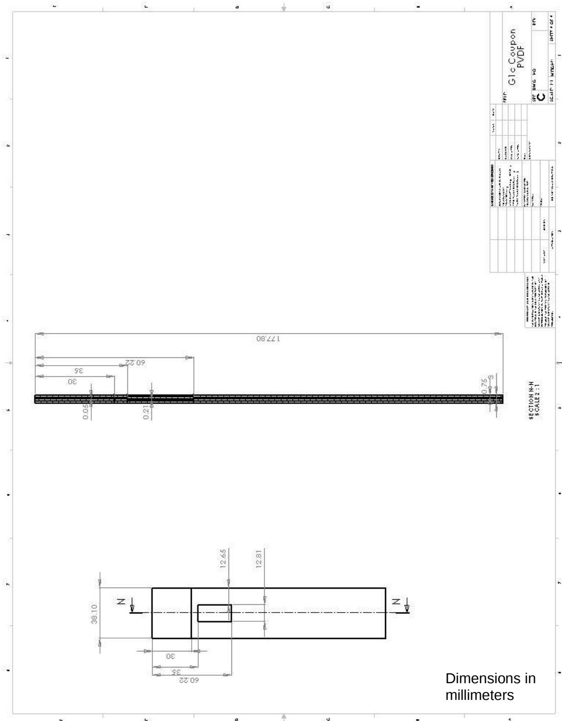
Figure 87, Dimensions of the G1c coupons with embedded PVDF films.
