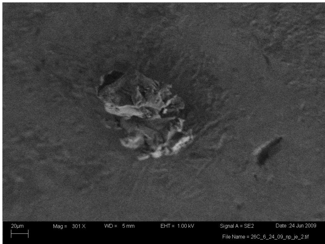
Figure 45. The surface of an embedded strain gage with no surface treatment, after failure. This was the largest resin particle found on the sensor surface.
