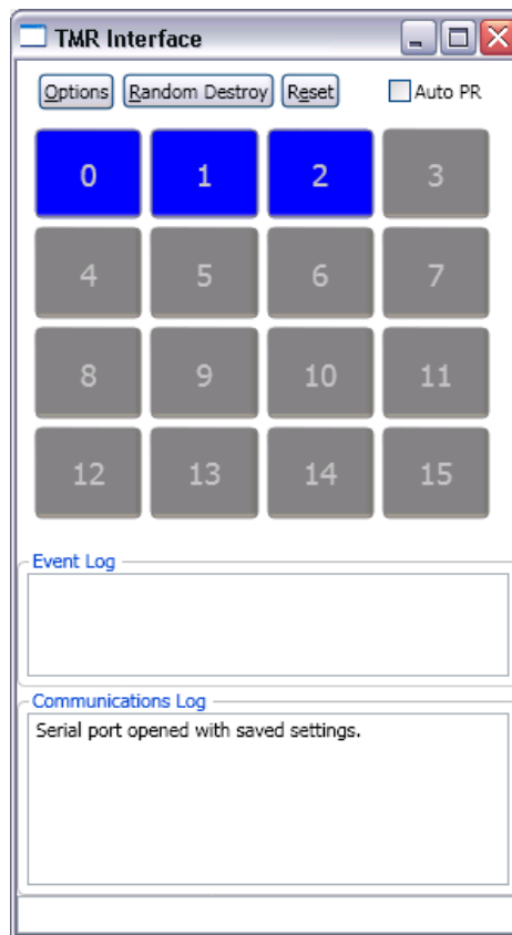
Figure 5.2: Screenshot of the 3+13 PicoBlaze GUI (Blue = Active, Red = Corrupted, Gray = Spare).
