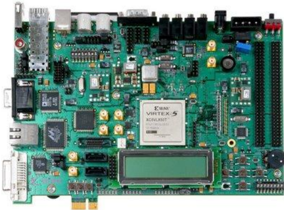
Figure 3.1: A Xilinx ML505 project board.
