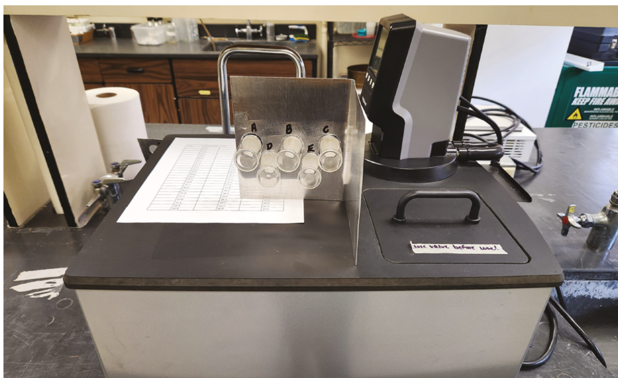
Fig. 2. Critical thermal minimum ( CTL_{min} ) ramping assay. Individual moth vials attached to aluminum sheet shown on top of programmable water bath.
