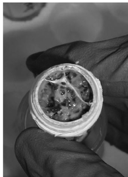
Fig. 3. Photos of SC-CO 2 extractor cartridges containing biofilm after exposure to PBS or SC-CO 2 . PBS exposed biofilm remained very moist whereas the biofilm samples processed with SC-CO 2 lost a portion of their water content and became visibly desiccated.
