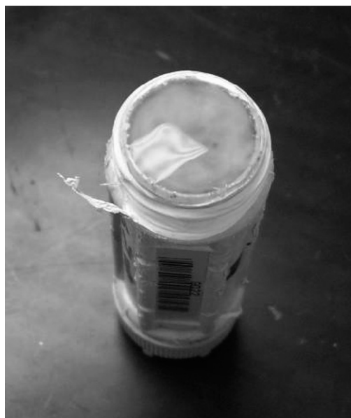
Fig. 3. Photos of SC-CO 2 extractor cartridges containing biofilm after exposure to PBS or SC-CO 2 . PBS exposed biofilm remained very moist whereas the biofilm samples processed with SC-CO 2 lost a portion of their water content and became visibly desiccated.
