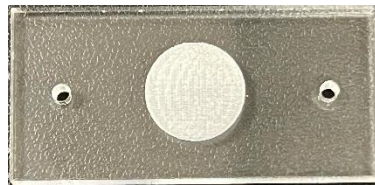
Figure B 1. Acrylic polish kit (Novus 7136) was applied to clean acrylic surfaces. A smooth surface was obtained by applying heavy scratch, fine scratch remover and plastic clean and shine, respectively.
