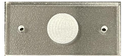
Figure B 1. Acrylic polish kit (Novus 7136) was applied to clean acrylic surfaces. A smooth surface was obtained by applying heavy scratch, fine scratch remover and plastic clean and shine, respectively.
