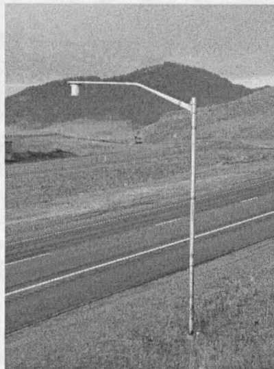
Figure 9. Down facing pyranometer over I-90
