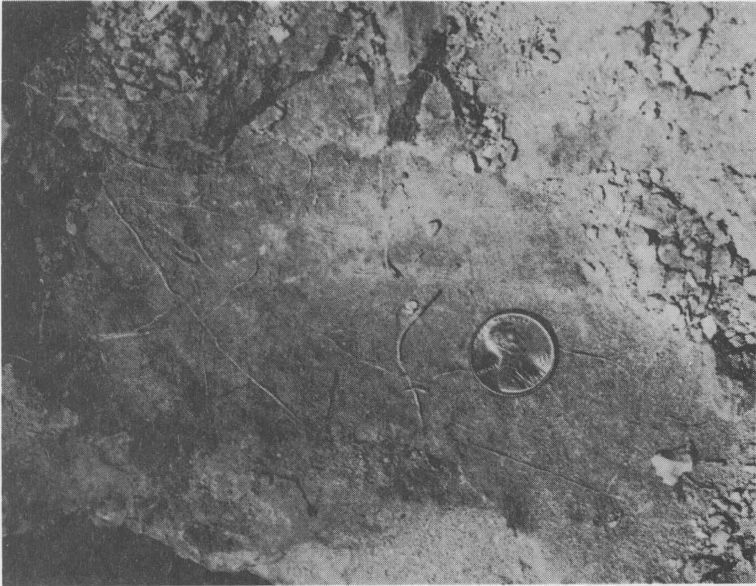
Figure 16. Compaction of the spoil surface before topsoil application can create a barrier to root penetration. The roots shown are flattened and horizontally-oriented on a compacted layer at 30 cm.
