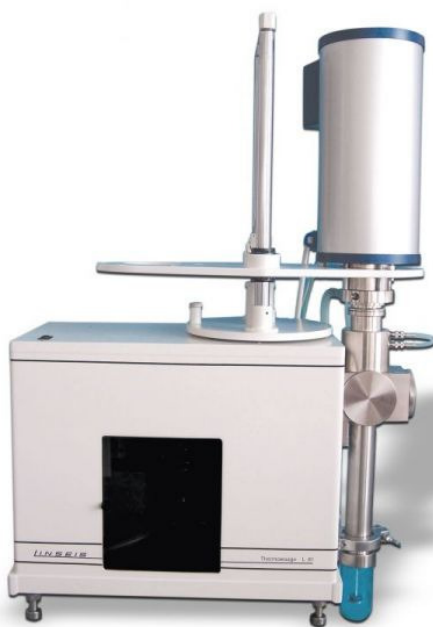
Figure 15: Linseis L81 Research Balance TG/DTA machine
