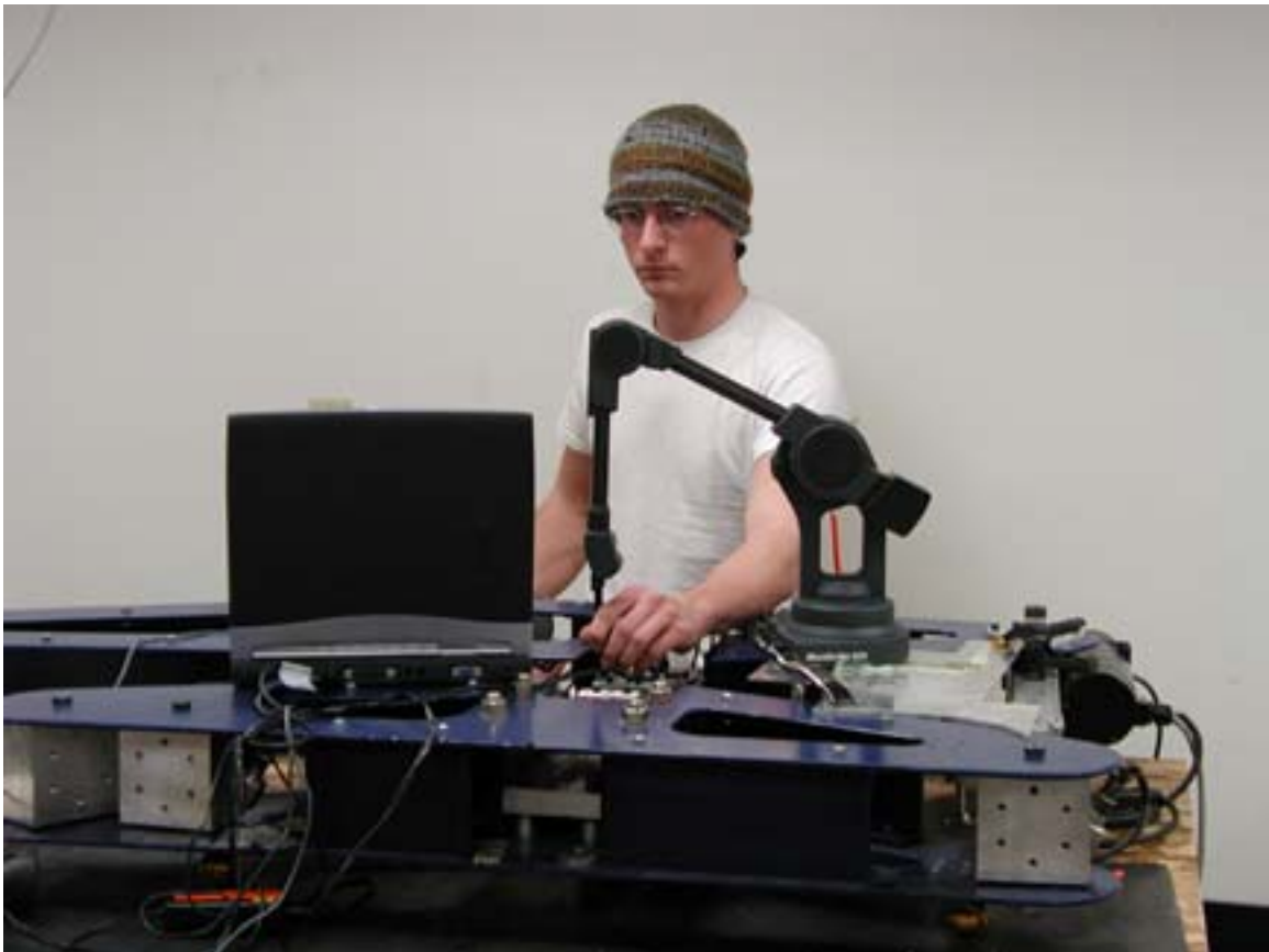
Figure 46. Using a digitization arm to measure the IPL.
