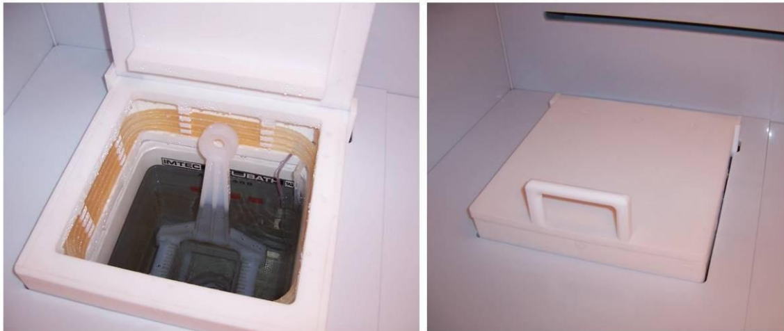
Figure 81: Pot used for TMAH bulk etching.
