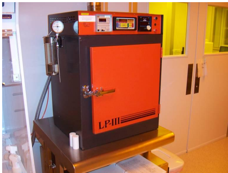
Figure 46: Vapor prime oven used to dehydrate wafers prior to spin-coating
