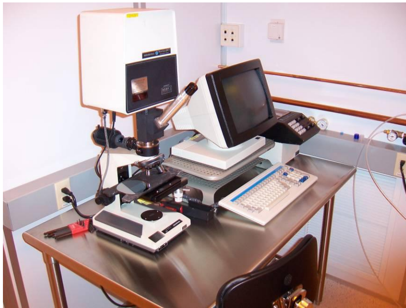
Figure 42: Nanospec equipment used to determine thicknesses of various films.
