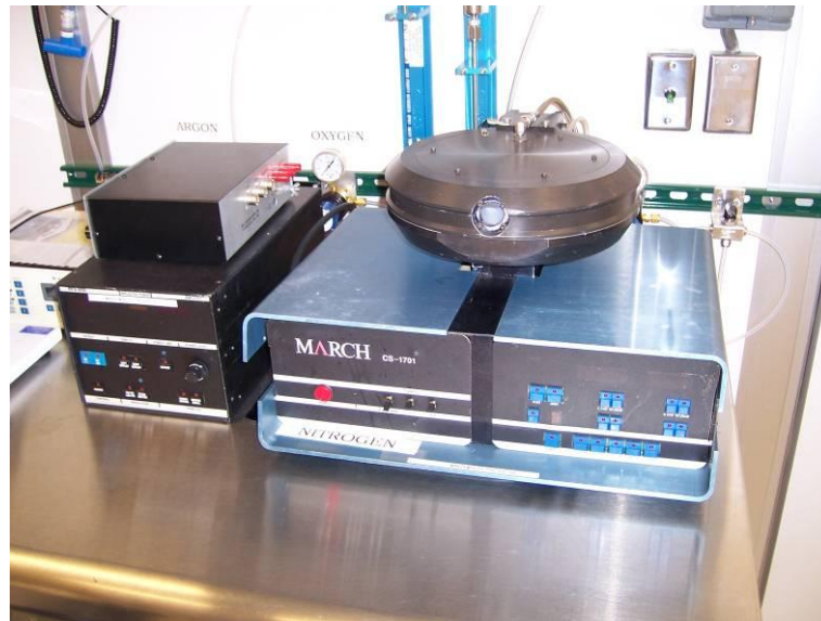
Figure 62: March Plasma Etcher used in plasma ashing process. The black box on the left is the RF power controller.
