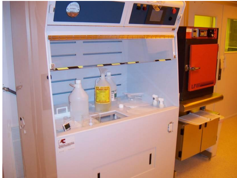
Figure 55: Wet bench used in development of the photoresist.
