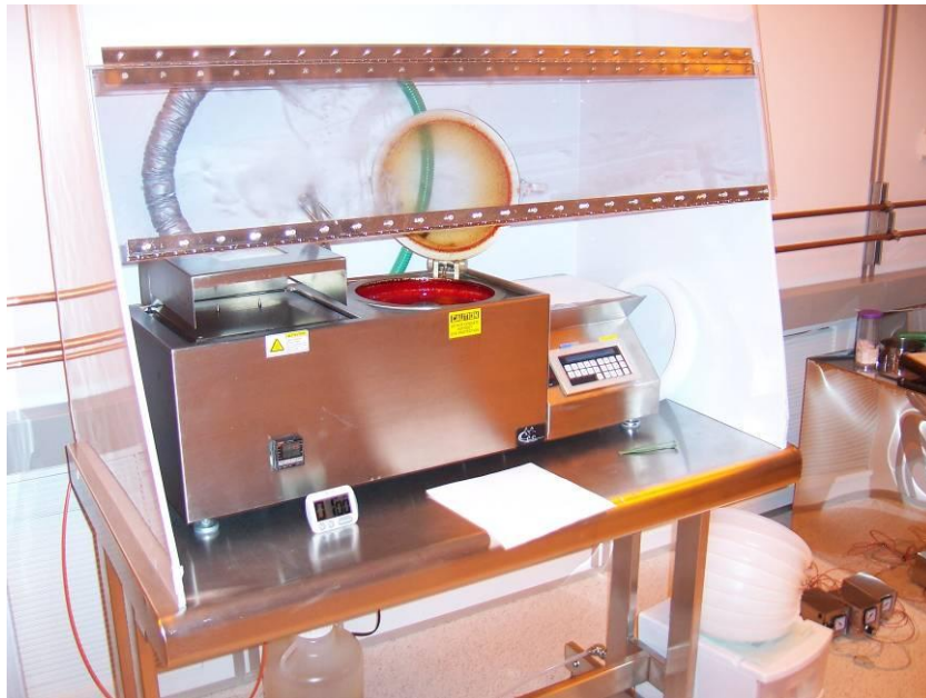
Figure 47: BREWER spin-coater and attached hotplate in fume hood.
