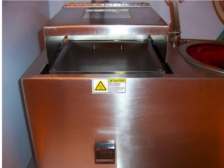
Figure 48: Hotplate used in wafer ‘baking’.
