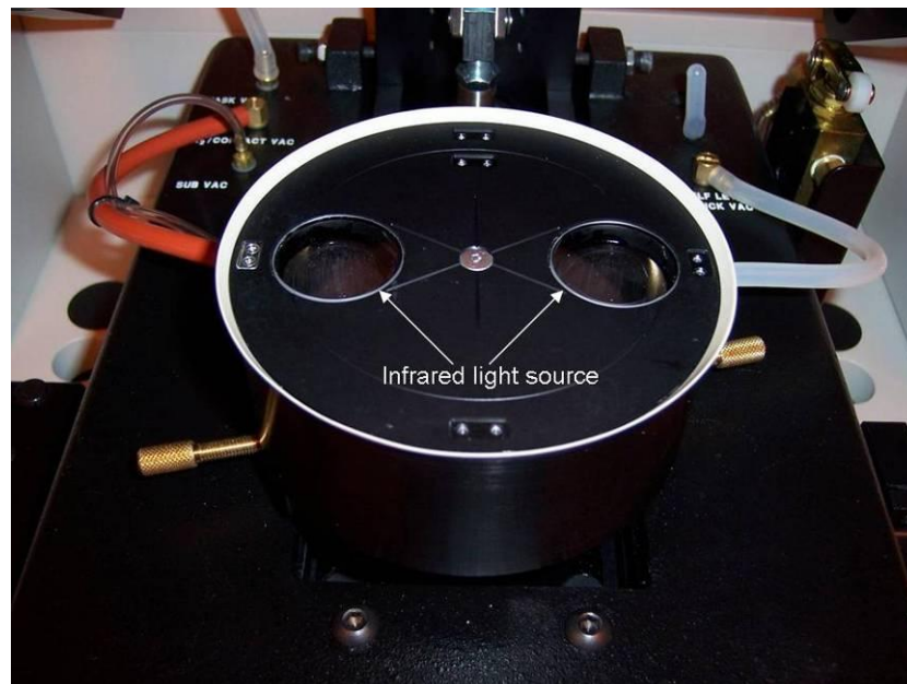
Figure 73: Infrared light sources on the ABM contact aligner vacuum chuck
