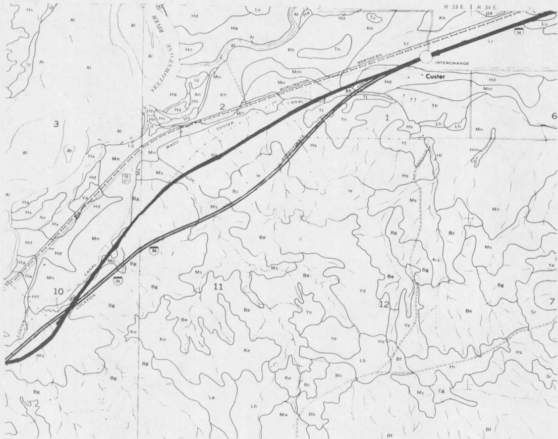
Figure 3. Actual location of I-94 through a portion of Yellowstone County (solid line) VS tentative I-94 location when soil survey was published (split parallel lines).
