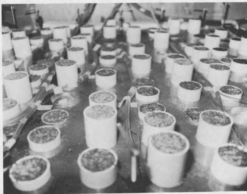
Figure 2. Thermogradient plate modified for seedling emergence studies at different seeding depths.
