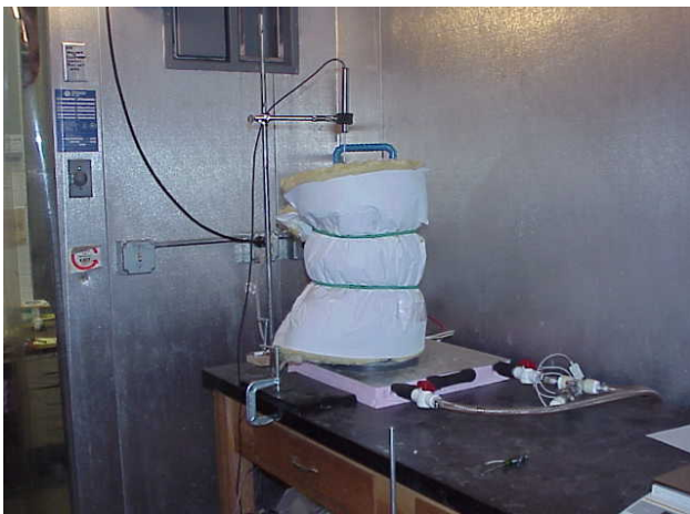
Figure 3.16: Photograph of insulated laboratory testing cylinder placed on the warm plate inside of the cold chamber.
