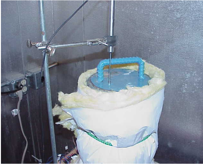
Figure 3.17: Photograph of steel cover plate and the linear variable displacement transducer (LVDT).
