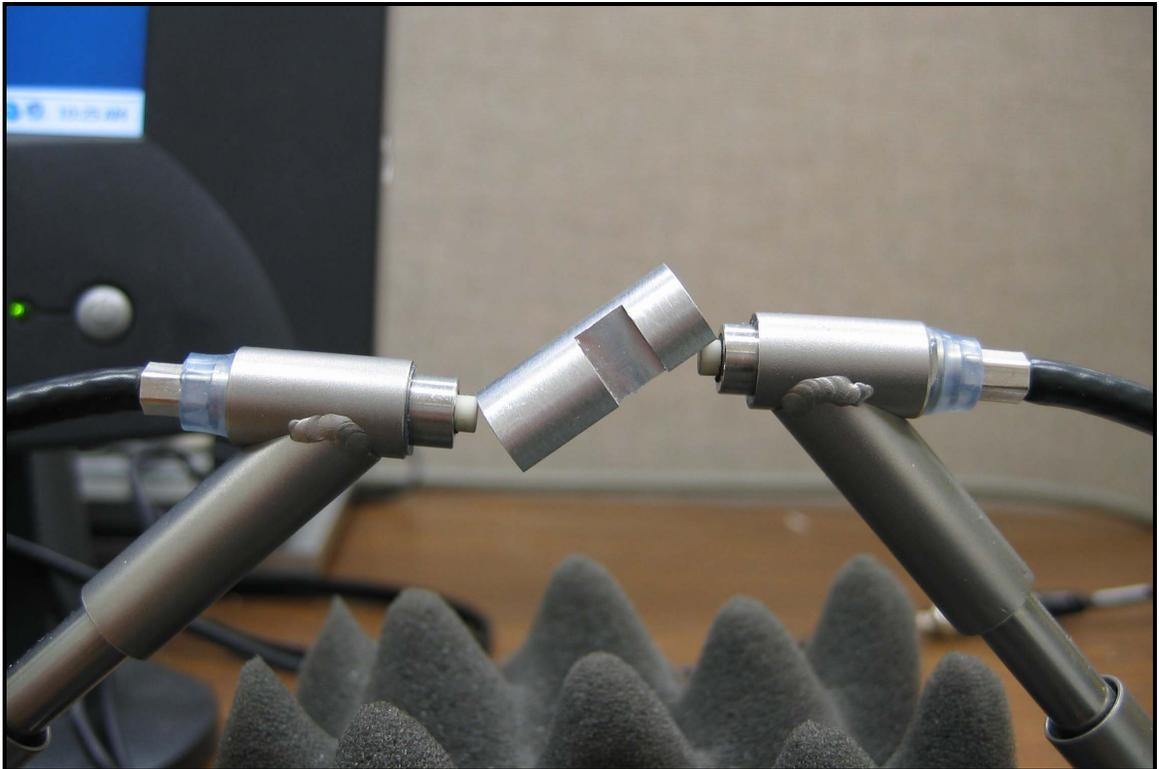
Figure 4.1 Experimental Setup. This image shows the Notch Cut sample held between the two DRS transducers.
