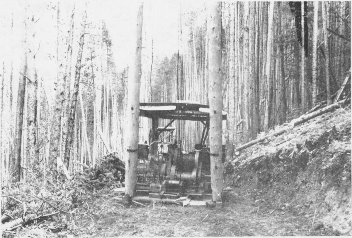
Figure 9. A homemade high lead skidder.
