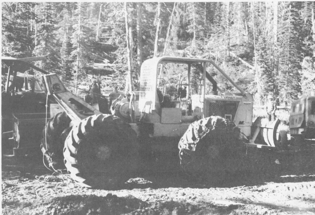
Figure 3. A Mountain Logger is a medium sized rubber-tired skidder.
