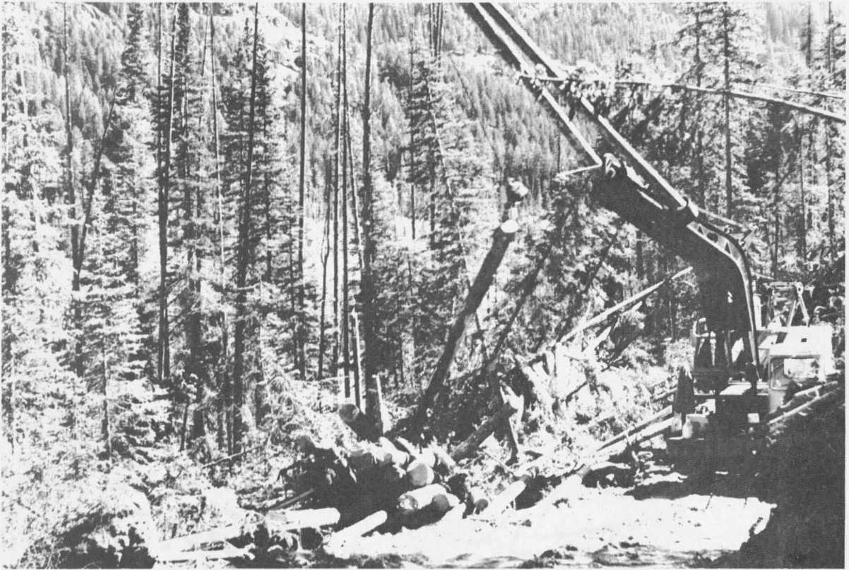
Figure 6. A combination 3/8 yard heel boom loader and jammer skidder mounted on a truck.
