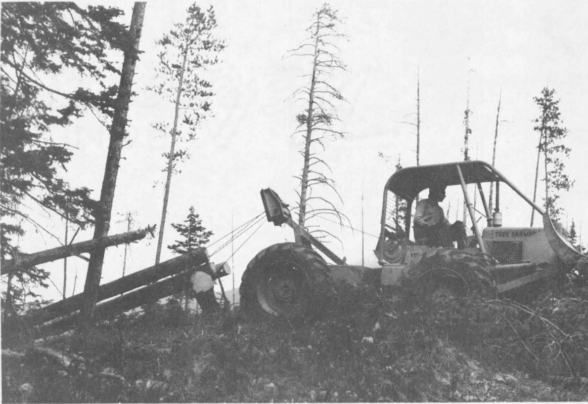
Figure 2. The Garrett Tree Farmer is a small rubber-tired skidder.
