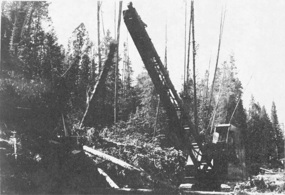
Figure 5. A 5/8 yard, steel boom jammer skidder mounted on tracks.
