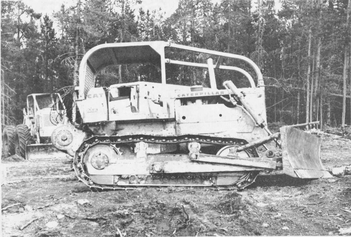
Figure 10. Crawler tractor with auxiliary equipment used for ground skidding.
