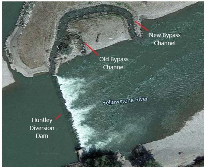
*Figure 2 - Huntley Diversion showing the old and new nature-like bypass channels. Image from Tupen (2020) and Google Earth.*
