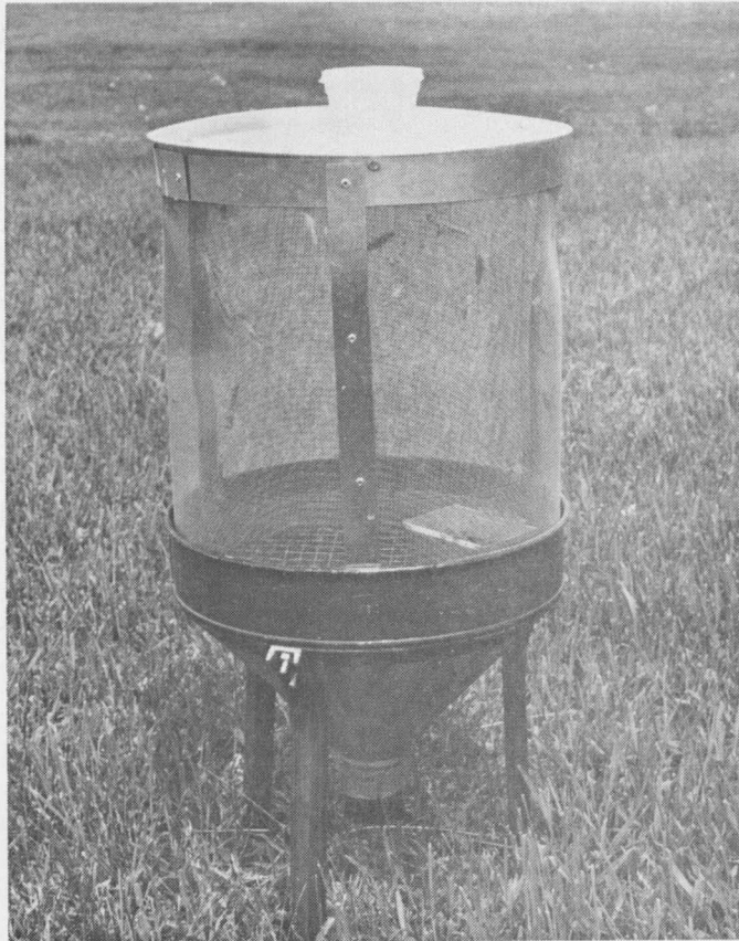
Fig. 3.--Cage (30 cm in dia X 35 cm high) used in the mass inoculation and rearing of grasshoppers for the production of spores of Nosema locustae for field tests.
