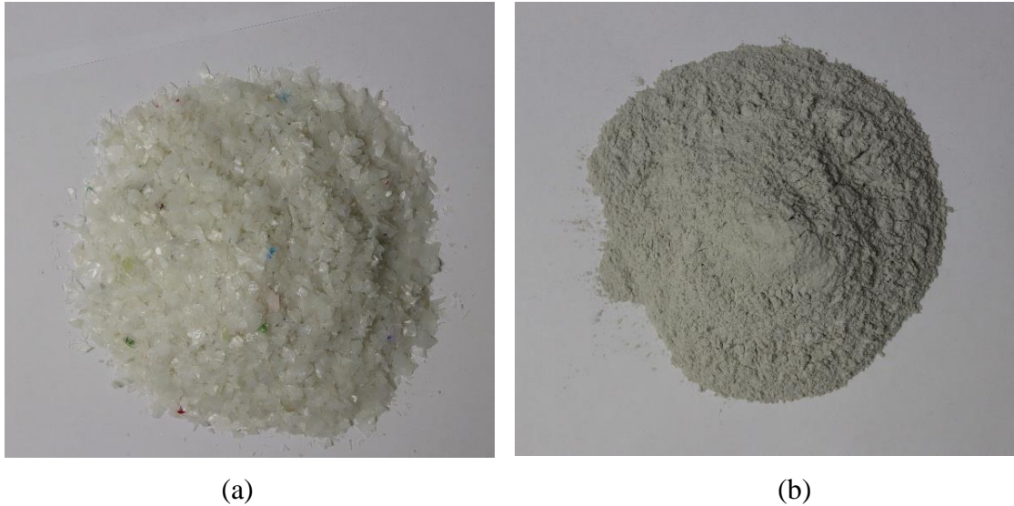
Figure 2.2: Materials used: (a) rHDPE; (b) talc filler.
