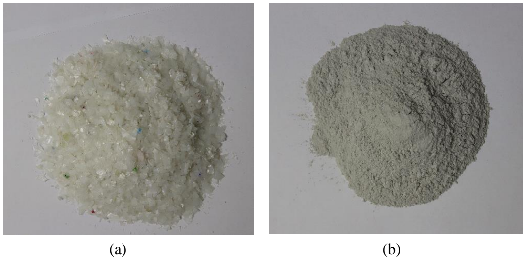
Figure 3.1: Materials used: (a) rHDPE; (b) talc filler.
