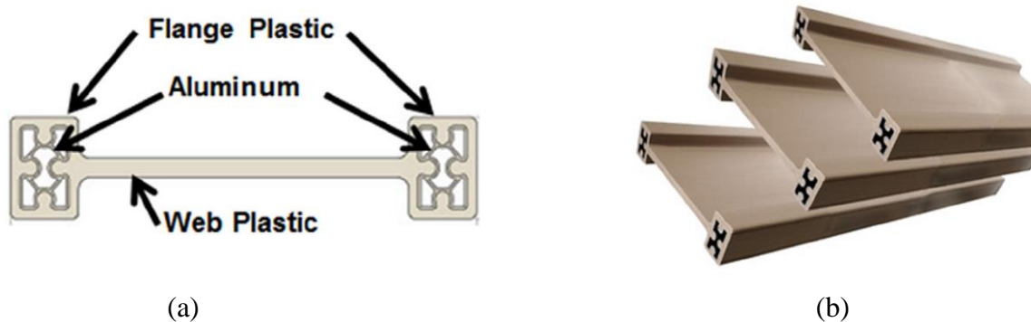
Figure 2.1: Plastic–aluminum composite I-beams: (a) cross-section; (b) length profile [24].
