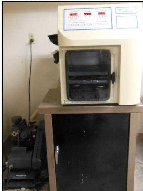
Figure 22. The shelf type vacuum freeze dryer system (Virtis EL-85) is shown. In the bottom left the vacuum pump can be seen.
