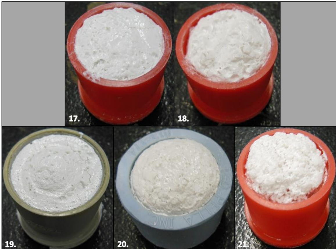
Figure 29. Results of the binder concentration study for 30% solids loading, where the sample numbers correlate with Table 4. All of the samples are in the green state prior to high temperature sintering.
