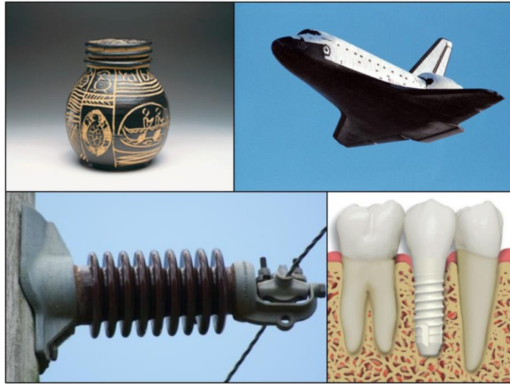
Figure 2. Examples of ceramic uses. Ceramic artwork from Montana artist Frances Sneska is shown in the upper left image (2). In the upper right image the silica fiber tiles on the space shuttle can be seen, black underside (4). The lower left image shows an electrical insulator used for transmission line, typically porcelain (5). Zirconia dental implants are depicted in the lower right image (3).
