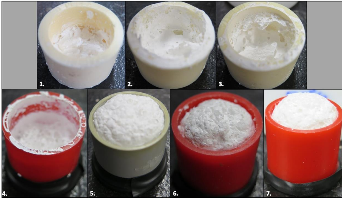
Figure 27. Results of the solids loading study, where the sample numbers correlate with Table 3. All of the samples are shown in the green state prior to high temperature sintering.
