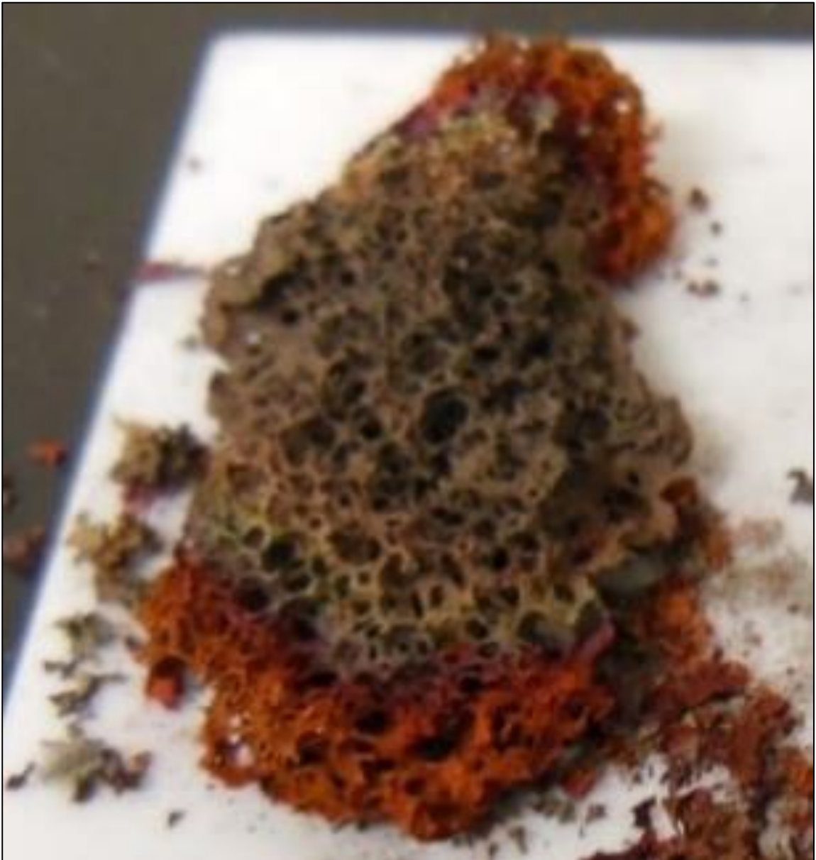
Figure 54. Copper foam synthesized using the freeze foaming process. Different oxidation states, indicated by different colors.
