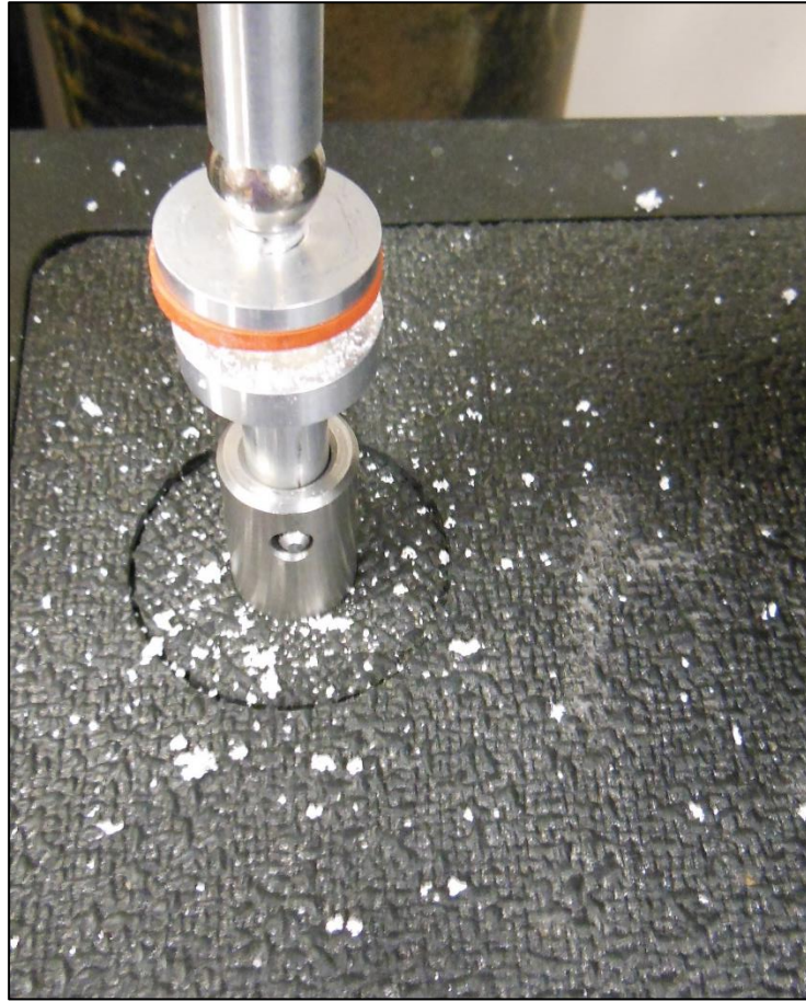
Figure 41. The effects of progressive failure resulted in ceramic foam chips flying off of samples during compression testing.
