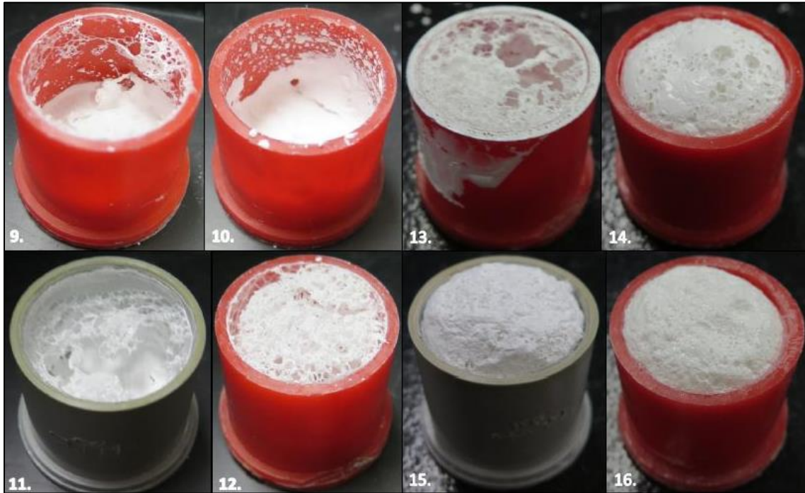
Figure 28. Results of the binder concentration study for 5% and 20% solids loading, where the sample numbers correlate with Table 4. All of the samples are in the green state prior to high temperature sintering.
