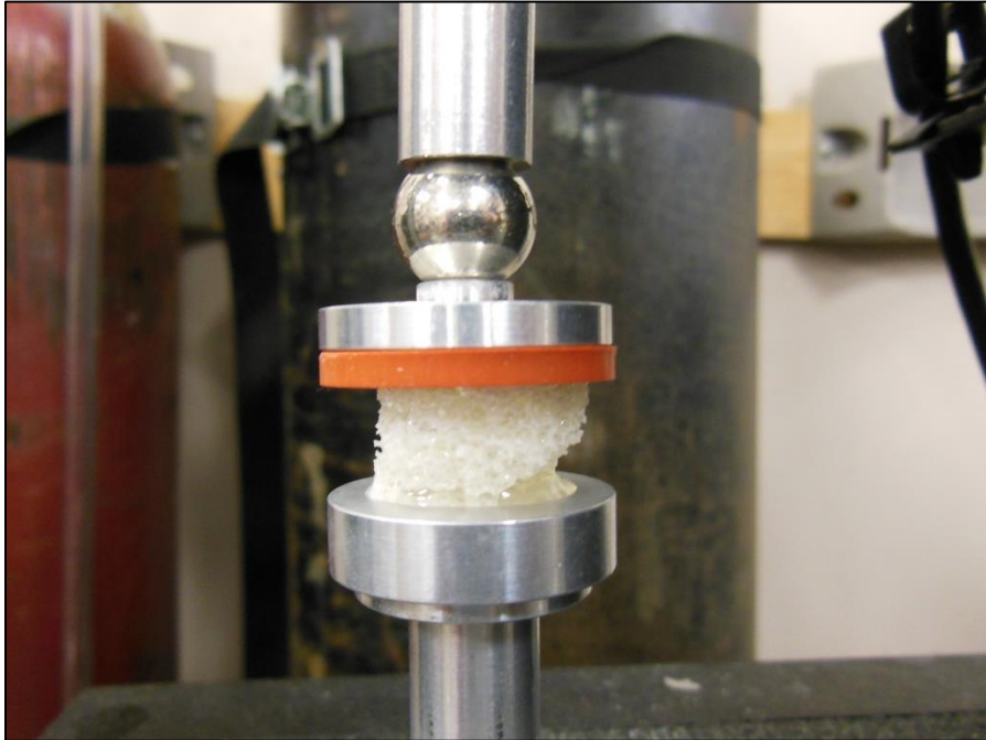
Figure 26. The compression test set up is shown. The metallic ball aligns the loading plate. The compliant silicon layer can be seen in orange, while the lower epoxy layer can be seen touching the support plate.
