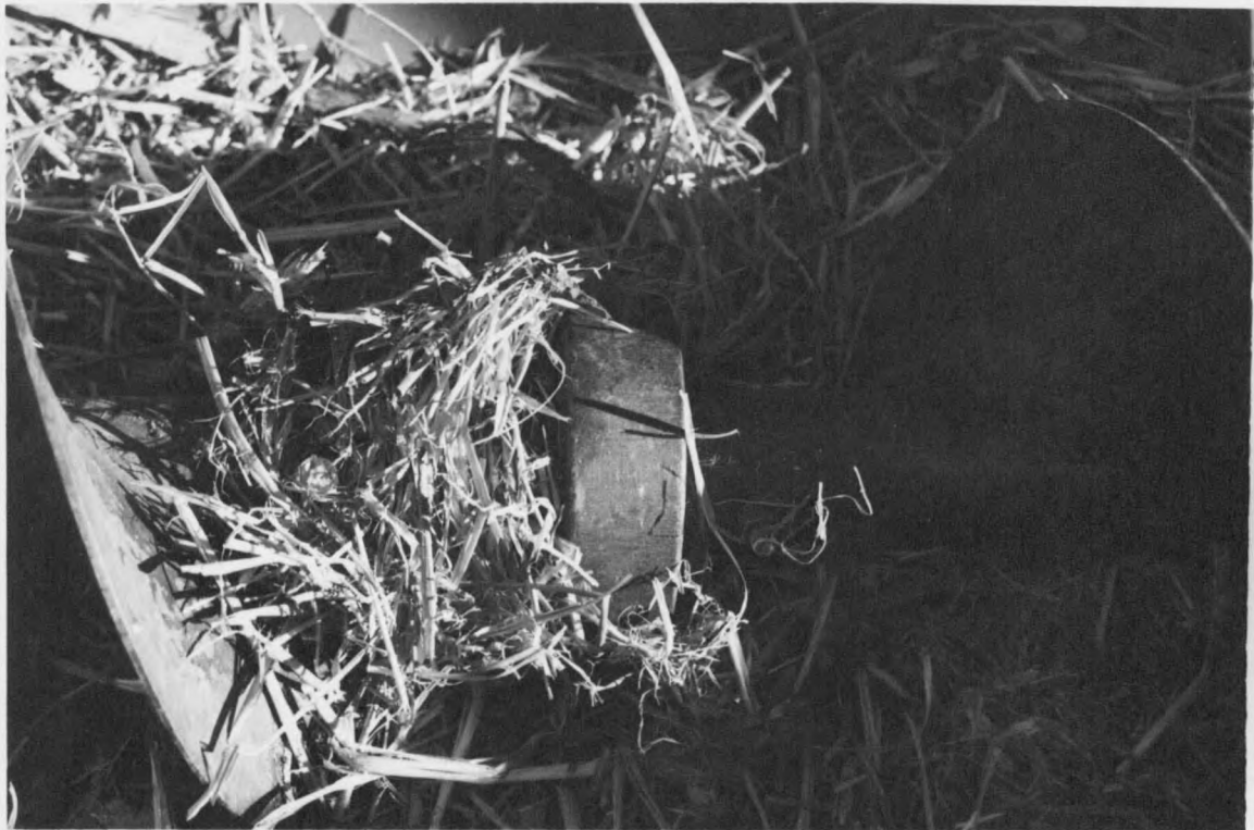
Figure 3. Binding problem around bearing.
