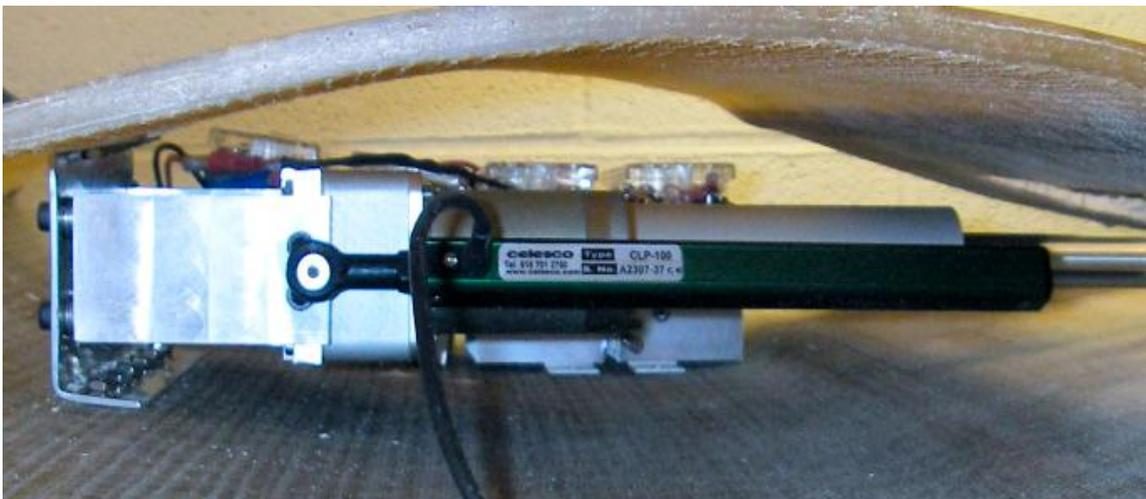
Figure 28: Rigid supports were added to eliminate the need for additional linkages to support the actuator and other hardware.
