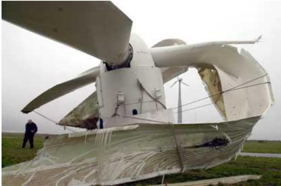
Figure 2: A wind turbine failure can be catastrophic, with devastating results. Tips of the blades can reach speeds in excess of 150 mph and pieces of the blades can be thrown over 1300 ft.
