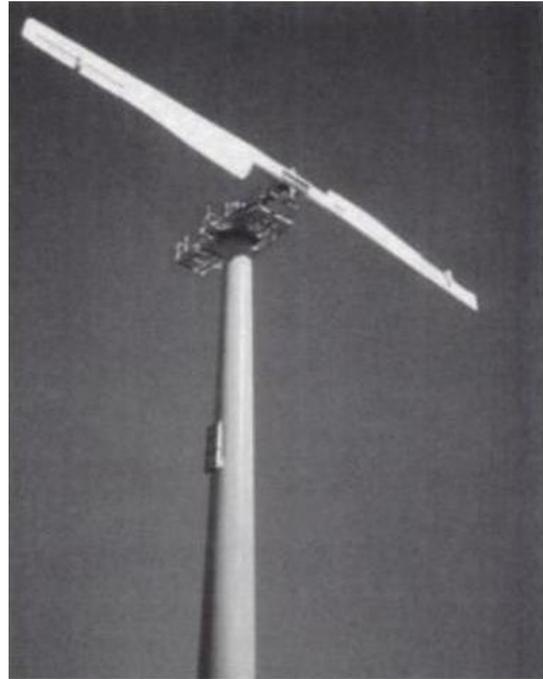
Figure 4: The North Wind 250 was developed in the early 1990s by Northern Power Systems. Its design incorporated an aileron style load control system.
