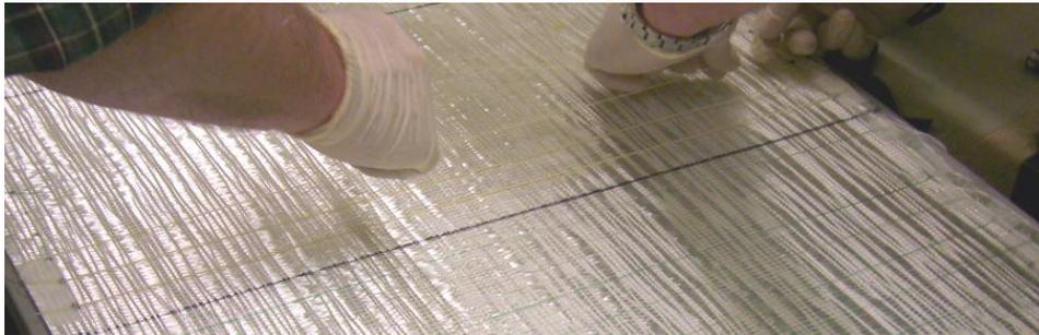
Figure 56: Damage to the optical fiber during handling and manufacturing is a major concern in the survivability of FOSs.
