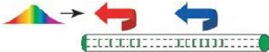
Figure 55: With a WDM interrogator each FBG reflects only its individual Bragg Wavelength, by monitoring that wavelength, the interrogator is capable of differentiating the individual FBGs.
