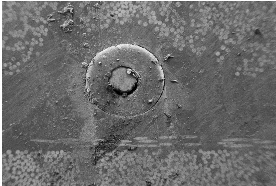
Figure 61: Embedding an optical fiber in a laminate results in a large resin pocket surrounding the optical fiber, which can compromise the strength of the laminate.
