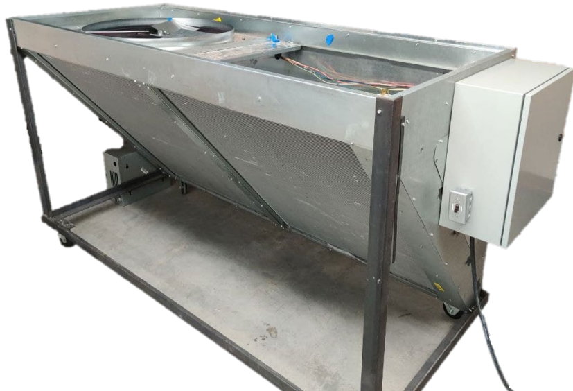
Figure 20. Condenser unit test stand used for collecting coil pressure differentials, velocities, and motor power data.
