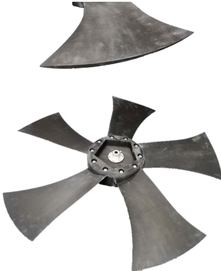
Figure 39. 3D printed fan (top) and assembly (bottom).
