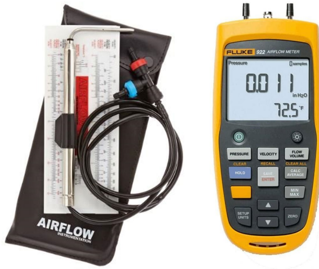
Figure 42. Alnor Telescoping Pitot Tube (Left); Fluke 922 Airflow Meter (Right).
