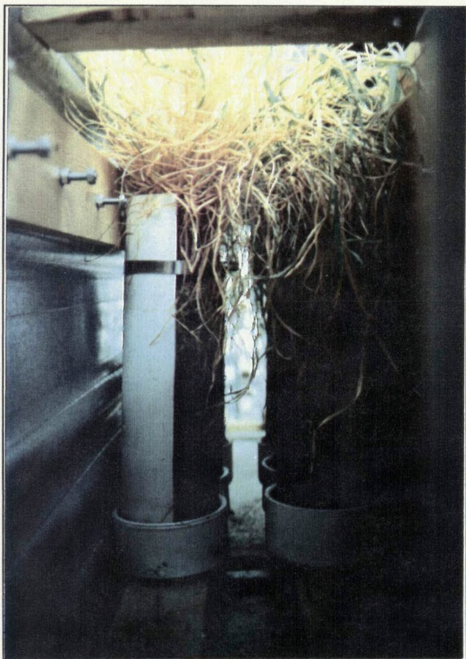
Figure 4. Positioning of samples in streamflow simulator.
